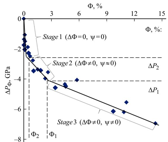
Figure 3. Staging of destruction depending on  $\Delta P_\Phi(\Phi)$  at strain amplitudes 0.25–0.35%.
