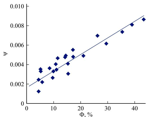
Figure 4. The dependence of micro-damage  $\psi$  on the volume fraction of  $\alpha'$ -martensite  $\Phi$ .
