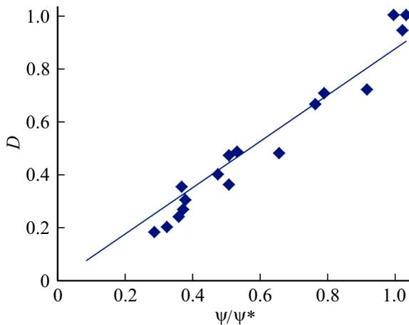
**Figure 6.** The relationship of the damage  $D$  with the value  $\psi/\psi^*$ .
