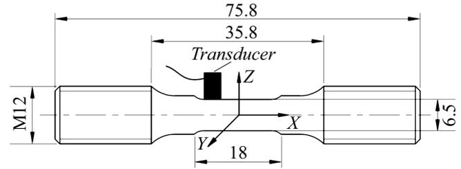
**Figure 1.** The shape of the fatigue test specimen and the transducer setup diagram
