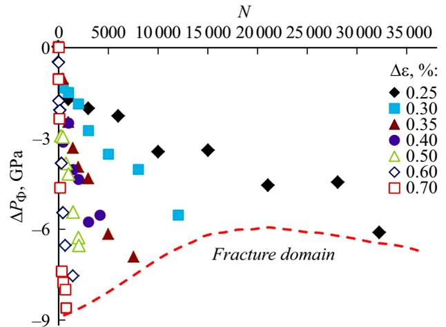
Figure 2. Dependence of the parameter change  $P_\Phi$  on the number of loading cycles.
