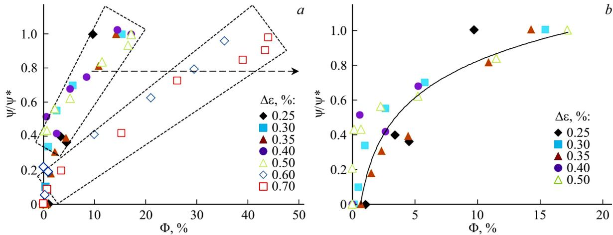
**Figure 5.** Dependence  $\psi/\psi^*$  on the change of the volume fraction of martensite  $\Phi$  (a), for strain amplitudes from 0.25 to 0.5% (b).
