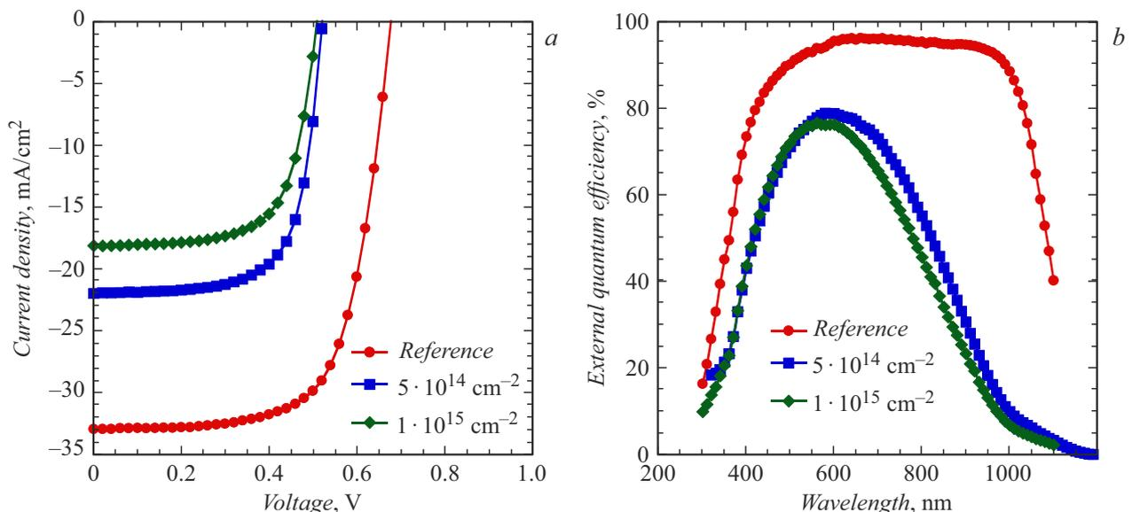
**Figure 2.** Current-voltage curve (a) and quantum efficiency (b) of samples with *n*-Si ( $n = 3 \cdot 10^{15} \text{ cm}^{-3}$ ): initial and after irradiation with doses of  $5 \cdot 10^{14}$  and  $1 \cdot 10^{15} \text{ cm}^{-2}$ .
