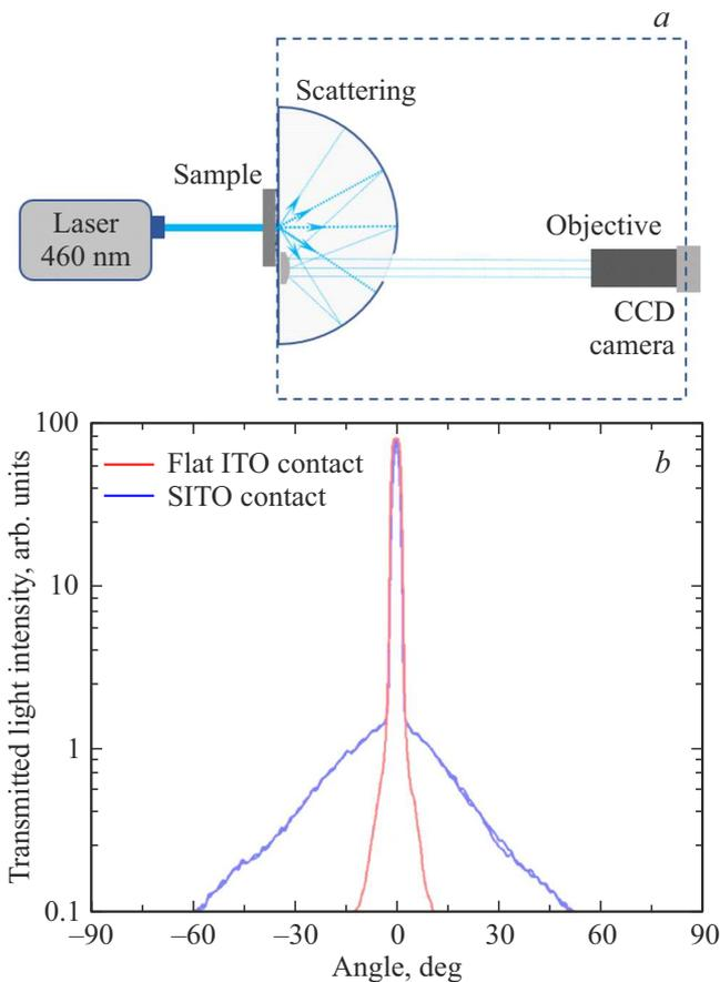
**Figure 2.**  $a$  — measurement scheme;  $b$  — directional patterns of light scattering on samples.
