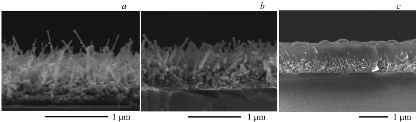
**Figure 1.** SEM image of film  $\text{Al}_2\text{O}_3$  with thickness  $a$  — 10 nm,  $b$  — 20 nm and  $c$  — 300 nm deposited on top of a nanostructured layer ITO.
