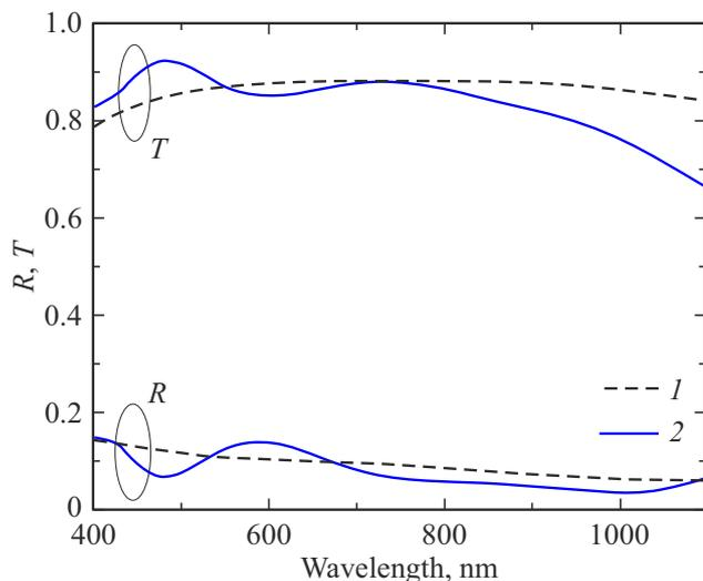
**Figure 3.** Reflection and transmission spectra of ITO film obtained in argon atmosphere (1) and ITO film obtained in oxygen-containing atmosphere (2).
