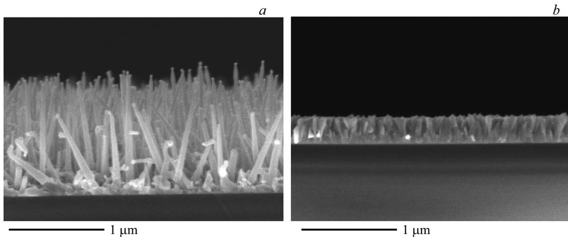
**Figure 1.** SEM image of ITO film grown: *a* — in oxygen-free atmosphere, *b* — in oxygen-containing atmosphere.
