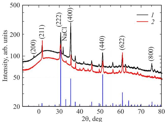
**Figure 2.** Diffraction curves of film deposited at temperature of 550°C and obtained: 1 — in argon atmosphere, 2 — in argon and oxygen atmosphere. Blue color indicates the bar diagram of the ICDD card, PDF-2, No. 00-044-1087, release 2014.
