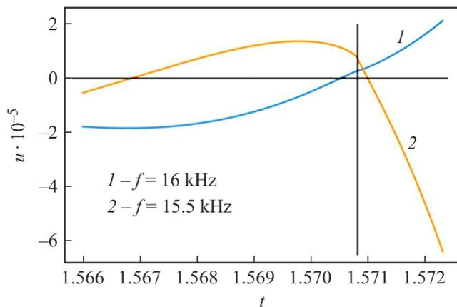
**Figure 2.** Calculations in the vicinity of the critical moment. At the critical moment (shown by the vertical line), the behavior of the solutions differs in the sign of the boundary acceleration: for a collapsing bubble, the acceleration is directed inwards, while for an expanding — outwards.
