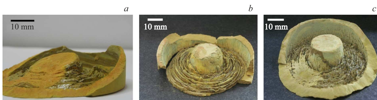
Figure 2. Photo of target residues after obtaining ZnSe nanopowders at Ar atmospheric pressure ( p = 100 kPa, (a, b)) and overpressure ( p = 300 kPa, (c)). Laser radiation generation mode — repetitively-pulsed (a) and continuous (b, c).
