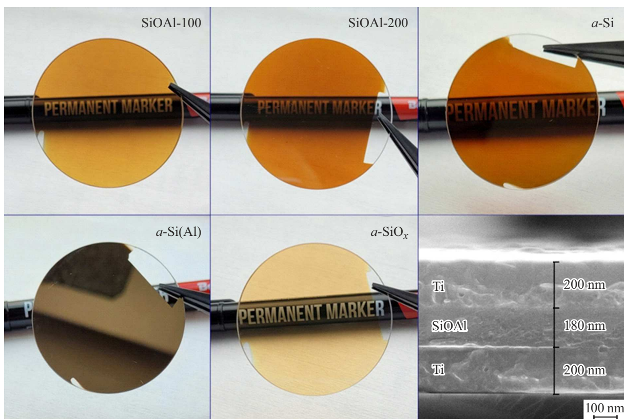
Figure 2. Films Si@O@Al, a -Si, a -Si 0.9 (Al 0.1 ) and a -SiO 0.8 on a substrate of fused quartz and SEM, an image of a chip of the Ti–Si@O@Al–Ti structure on a silicon substrate. The elemental composition of the films is shown in Figure and in Table. 2.
