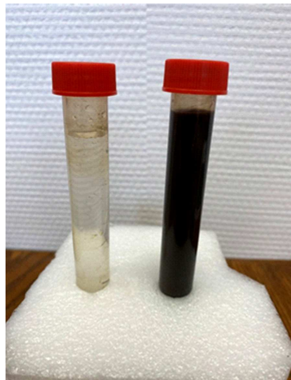
Figure 10. The main heat carriers of LTS2: water (left) and water + 2% Cu_xO_y (right) after three months of storage.
