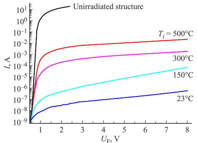
**Figure 1.** Static direct volt-ampere characteristics of structures irradiated with protons with an energy of 15 MeV at a dose of  $10^{14} \text{ cm}^{-2}$  at four irradiation temperatures  $T_i$ . The upper curve corresponds to the volt-ampere characteristic of the non-irradiated sample [21].
