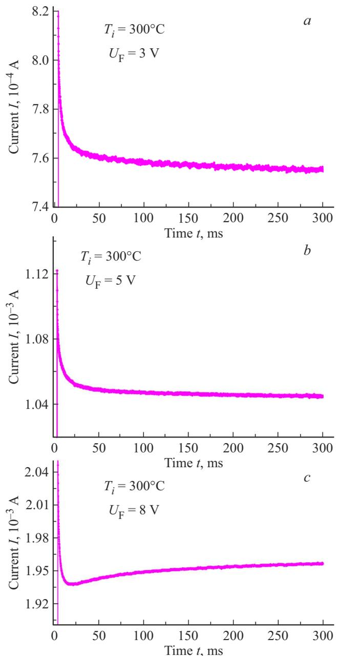
**Figure 4.** A long-term transient process of establishment of a stationary state in case of application of pulse voltage with an amplitude of  $U_F$  is applied to a sample irradiated with a dose of  $\Phi = 10^{14} \text{ cm}^{-2}$  at  $T_i = 300^\circ\text{C}$ . Voltage  $U_F$ , V: *a* — 3, *b* — 5, *c* — 8. Voltage rise rate  $dU_F/dt = 2 \cdot 10^3$  V/s.
