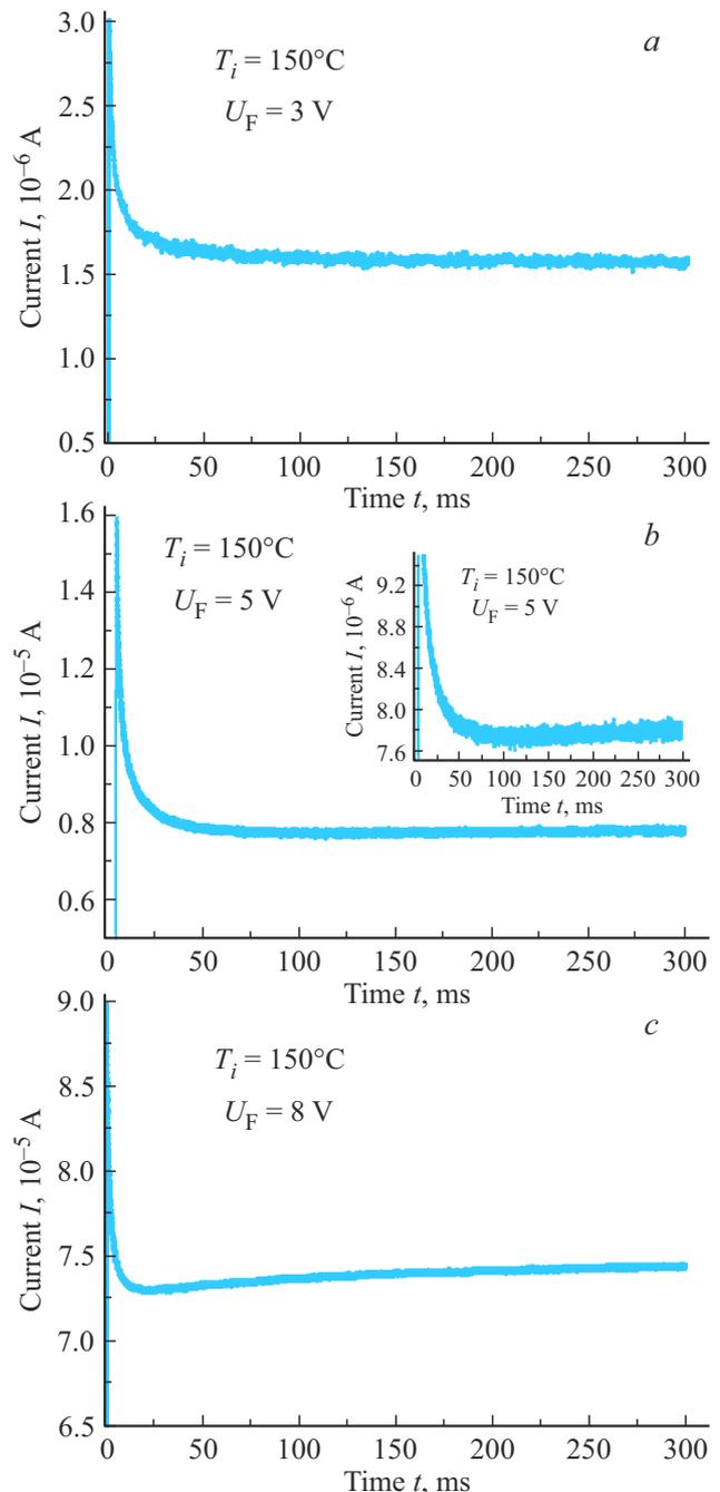
**Figure 3.** A long-term transient process of establishment of a stationary state in case of application of pulse voltage with an amplitude of  $U_F$  to a sample irradiated with a dose of  $\Phi = 10^{14} \text{ cm}^{-2}$  at  $T_i = 150^\circ\text{C}$ . Voltage  $U_F$ , V: *a* — 3, *b* — 5, *c* — 8. The dependence  $I(t)$  is shown with a high resolution of current  $I$  in the box to Figure 3, *b*. Voltage rise rate  $dU_F/dt = 2 \cdot 10^3 \text{ V/s}$ .
