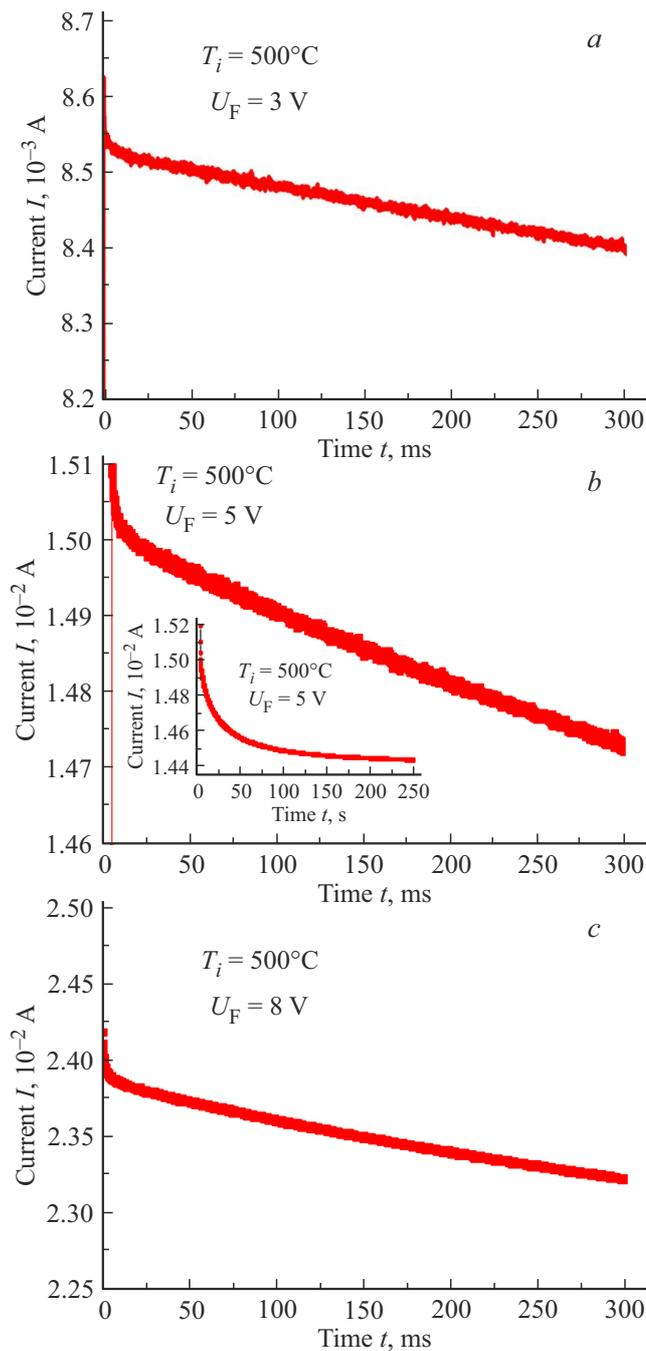
**Figure 5.** A long-term transient process of establishment of a stationary state in case of application of pulse voltage with an amplitude of  $U_F$  to a sample irradiated with a dose of  $\Phi = 10^{14} \text{ cm}^{-2}$  at  $T_i = 500^\circ\text{C}$ . Voltage  $U_F$ , V: *a* — 3, *b* — 5, *c* — 8. The dependence  $I(t)$  is traced in the time range of hundreds of seconds in the box to Figure 5, *b*. Voltage rise rate  $dU_F/dt = 2 \cdot 10^3 \text{ V/s}$ .
