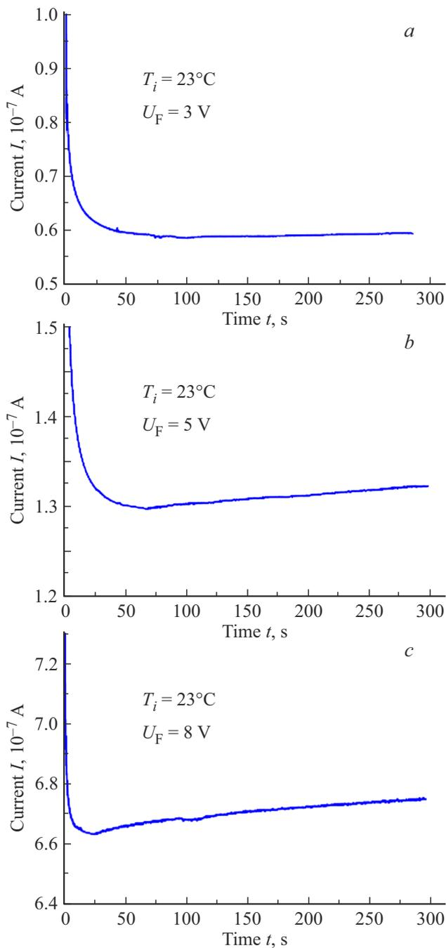
**Figure 2.** A long-term transient process of establishment of a stationary state in case of application of pulse voltage with an amplitude of  $U_F$  to a sample irradiated with a dose of  $\Phi = 10^{14} \text{ cm}^{-2}$  at  $T_i = 23^\circ\text{C}$ . Voltage  $U_F$ , V: *a* — 3, *b* — 5, *c* — 8. Voltage rise rate  $dU_F/dt = 10^2 \text{ V/s}$ .
