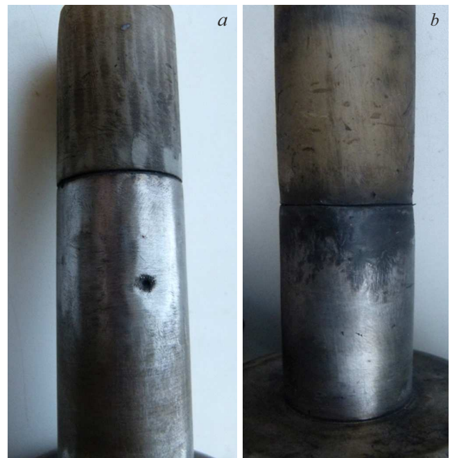
Figure 4. Photographs of the electrode surface. a — experiment without the EEOS foil in the gap of the gating, b — experiment with the EEOS foil in the CS gap
