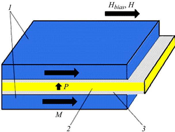
**Figure 2.** Schematic representation of the DOE structure: 1 — magnetostriction layer, 2 — piezoelectric layer, 3 — thin conductor (Ag) layer. The arrows show the directions of magnetization  $M$ , polarization  $P$ , sub-magnetization field  $H_{bias}$ , and alternating magnetic field  $H$ .
