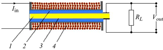
**Figure 1.** Schematic diagram of the gyator: 1 — piezoelectric layer, 2 — magnetostriction layers, 3 — thin silver layer, 4 — inductance coil. Input current  $I_{in}$ , output voltage  $V_{out}$ , load resistance  $R_L$ .
