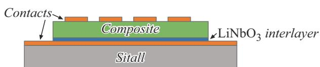
Figure 1. Topology of the experimental samples M/NK/D/M/M.
