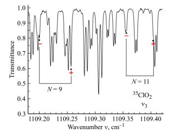
Small fragment of the experimental spectrum of a ClO<sub>2</sub> molecule from [37]. "Forbidden"  $\Delta k = -2$  transitions are denoted by dark circles. The experimental conditions are as follows: spectral resolution — 0.0015 cm<sup>-1</sup>; number of scans — 400; radiation source — Globar; detector — MCT313; KBr beam splitter; optical path length — 0.23 m; aperture — 1.15 mm; temperature — 22.0±0.3°C; pressure — 100 Pa; CO<sub>2</sub> and H<sub>2</sub>O lines were used for calibration.
