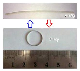
Figure 6. Implementation of the TWSME in amorphouscrystalline composite made of rapidly quenched alloy  $Ti_{50}Ni_{25}Cu_{25}$ .
