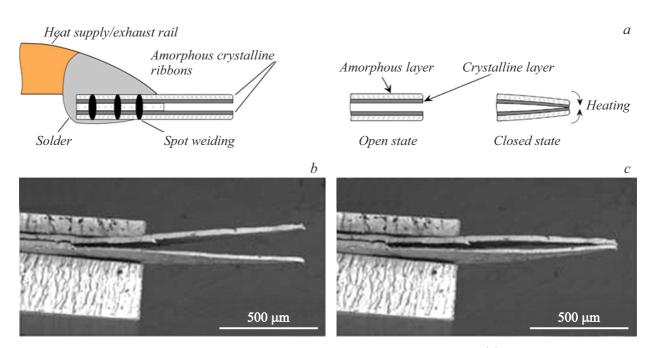
**Figure 8.** Schematic representation of microtweezers based on a composite ribbon with TWSME (a). SEM image of microtweezers in open (b) and closed (c) states.
