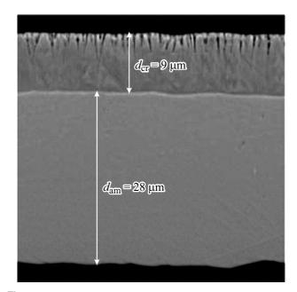
Figure 5. Representative electron microscopic image of the cross section of the amorphous-crystalline ribbon of alloy  $Ti_{50}Ni_{25}Cu_{25}$ .
