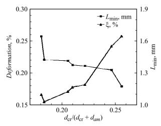
**Figure 7.** Deformation  $\varepsilon$  and minimum length of ribbon  $L_{\min}$ , which ensures movement of the free end $\Delta = 60 \,\mu$ m vs. thickness ratio  $d_{\rm cr}/(d_{\rm cr} + d_{am})$ .
