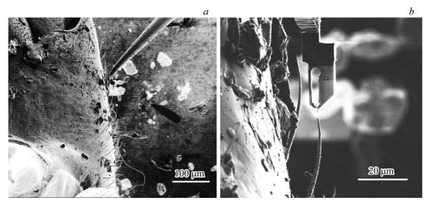
**Figure 1.** a — selection of an individual sensilla of a mosquito *C. pipiens* using nanotweezers with SME mounted on a tungsten microneedle, which is positioned by Omniprobe nanomanipulator in the vacuum chamber of FEI Strata 201 FIB ion microscope (measuring ruler  $100 \mu$ m). b — capture and cutting of a fragment of the *C. pipiens* sensilla with an ion beam of FEI Strata 201 FIB microscope (measuring ruler  $20 \mu$ m).
