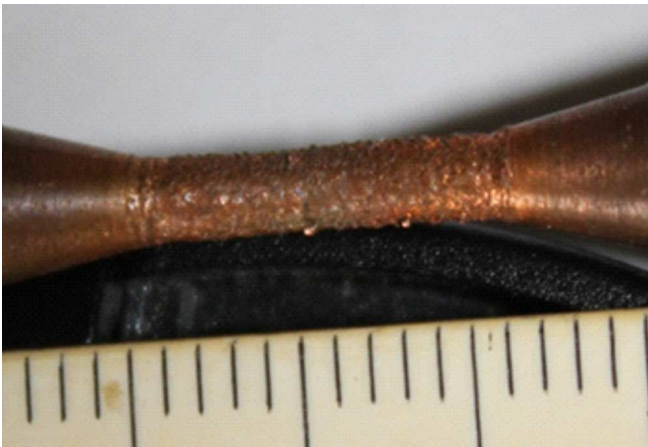
Figure 3. Photograph of copper sample after passing electric current. Amplitude of current pulse is 130 kA.
