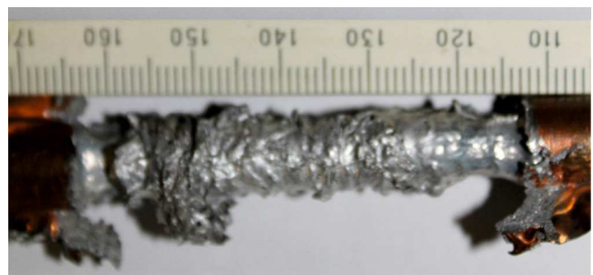
Figure 4. Photograph of duralumin sample. Current amplitude 300 kA, halfcycle 10 \mu\text{s} , attenuation coefficient 0.8, calculated instability wavelength 0.14 mm, and according to the sample image \sim 1 \text{ mm} .
