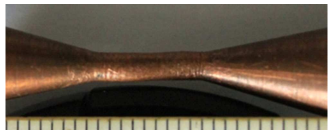
Figure 2. Photograph of special copper sample after passing pulsed electric current. Traces of instability in the form of transverse stripes are visible on the surface.
