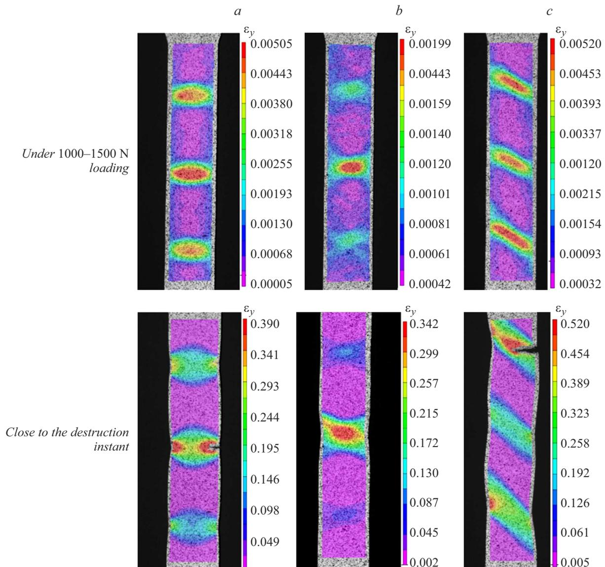
**Figure 3.** Fields of relative strains along the loading axis at different times, obtained in the system Vic 3D for samples with austenitic regions in the shape of round (*a*), square (*b*) and parallelogram (*c*).
