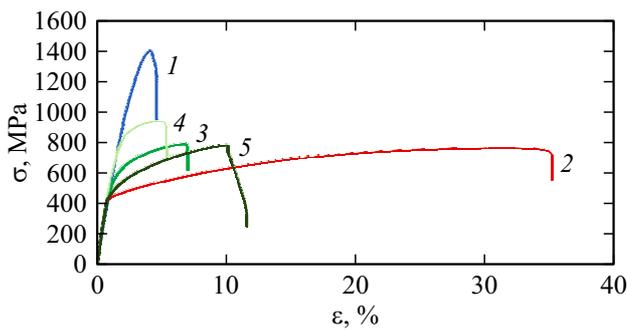
**Figure 2.** “Stress-strain” diagrams of the tested samples (1 — untreated, 2 — fully treated, 3 — in the shape of round, 4 — square, 5 — parallelogram).
