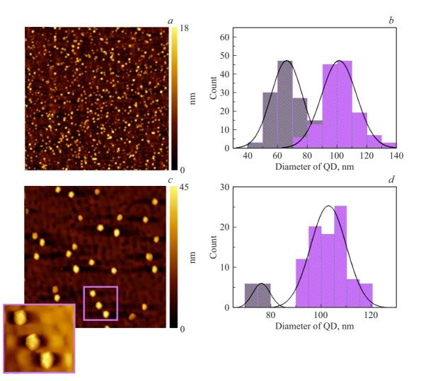
**Figure 1.** AFM-images  $(5 \times 5\mu m)$  of Si-surface after deposition of an InAs-layer with a thickness of 0.6 ML (*a*) and 1 ML (*c*). Bar charts of size distribution of InAs nanoislands formed after deposition of an InAs layer with a thickness of 0.6 ML (*b*) and 1 ML (*d*).
