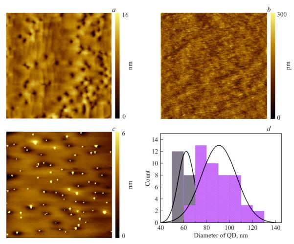
**Figure 2.** AFM-images  $(1 \times 1 \mu m)$  of the silicon buffer layer surface before (a) and after (b) thermal annealing. AFM-image  $(5 \times 5 \mu m)$  of InAs nanoislands formed on a smooth Si surface after deposition of an InAs layer with a thickness of 0.6 ML (s) and the corresponding bar chart of islands distribution by size (d).
