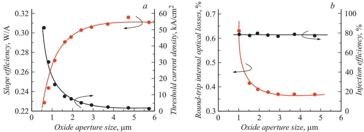
**Figure 2.** *a* — slope efficiency and threshold current density versus the oxide-confined aperture size for IC-VCSEL with an upper DBR based on eight SiO<sub>2</sub>/Ta<sub>2</sub>O<sub>5</sub> pairs; *b* — internal optical losses due to passing through the IC-VCSEL cavity versus the oxide-confined aperture size. The temperature is 20°C.
