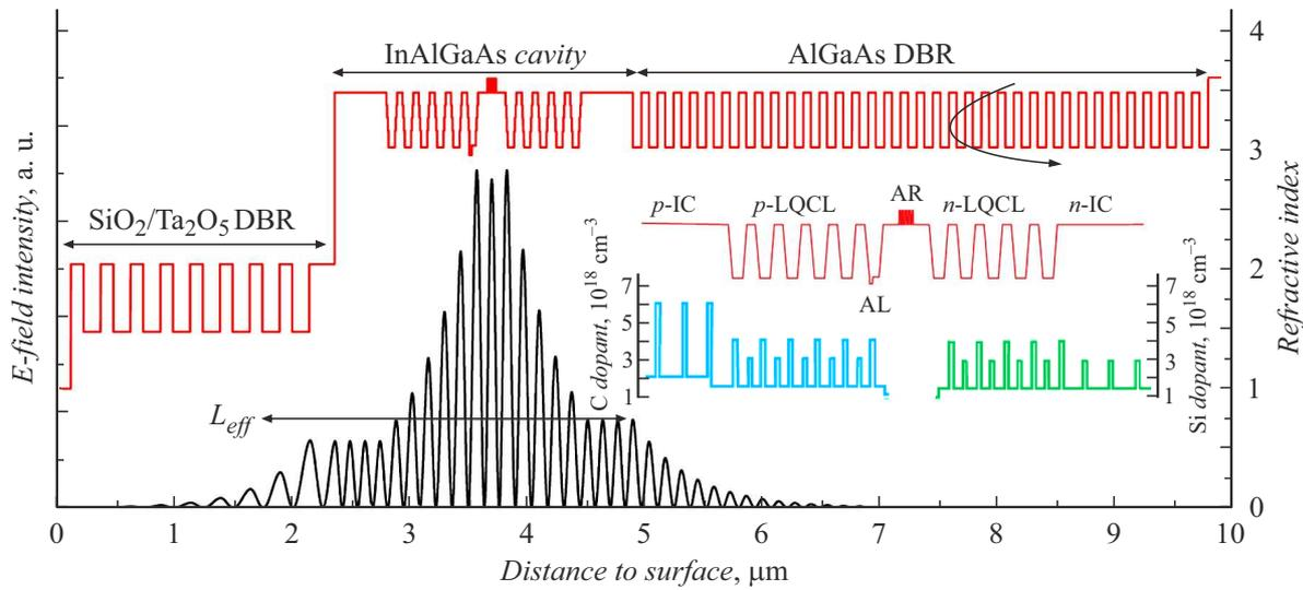
**Figure 1.** Longitudinal distribution of the standing wave electromagnetic field, refractive index and dopants (in the inset) in the IC-VCSEL microcavity. DBR — distributed Bragg reflector, IC — intracavity contact, LQCL — low-Q composite lattice, AR — active region, AL — aperture layer.
