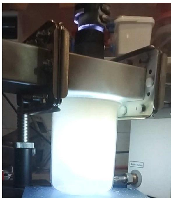
**Figure 1.** Illustration of the process of ZnO microstructure synthesis in the microwave plasma experiment.
