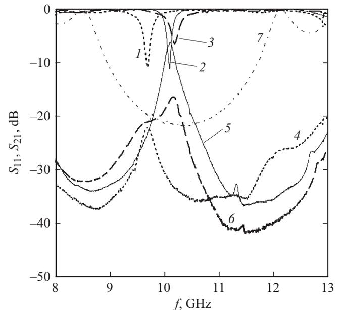
**Figure 3.** Experimental amplitude–frequency characteristics of reflection  $S_{11}(f)$  (1–3) and transmission  $S_{21}(f)$  (4–6) coefficients of the PC corresponding to different positions of the sample with a conducting nanolayer within the defect.  $L = 0$  (1, 4), 1.5 (2, 5), and 2.5 mm (3, 6). 7 — Amplitude–frequency characteristic of the transmission coefficient of the photonic crystal with no defects of periodicity.
