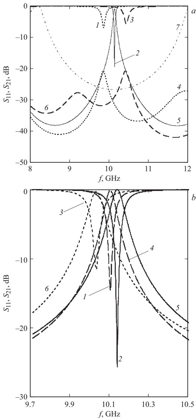
**Figure 2.** Calculated amplitude–frequency characteristics of reflection  $S_{11}(f)$  (1–3) and transmission  $S_{21}(f)$  (4–6) coefficients of the PC corresponding to different positions of the sample within the defect.  $L = 0$  (1, 4), 1.4 (2, 5), and 2.5 mm (3, 6). 7 — Amplitude–frequency characteristic of the transmission coefficient of the photonic crystal with no defects of periodicity. *a* — With a conducting nanolayer; *b* — without a conducting nanolayer.
