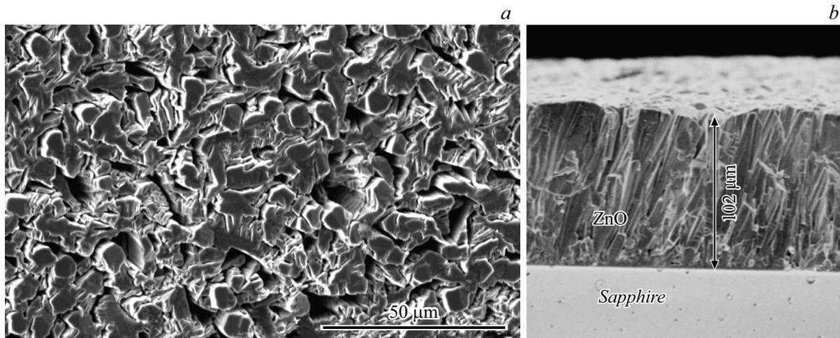
**Figure 1.** Photomicrographs of the ZnO film structure. *a* — Surface; *b* — transverse section.
