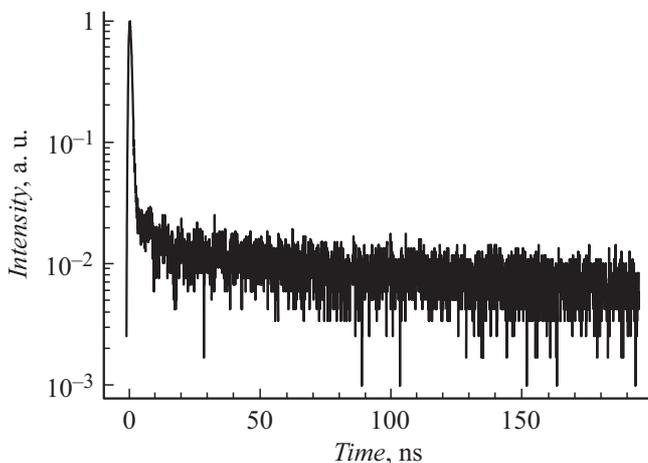
**Figure 3.** Decay kinetics of exciton luminescence of a ZnO film.
