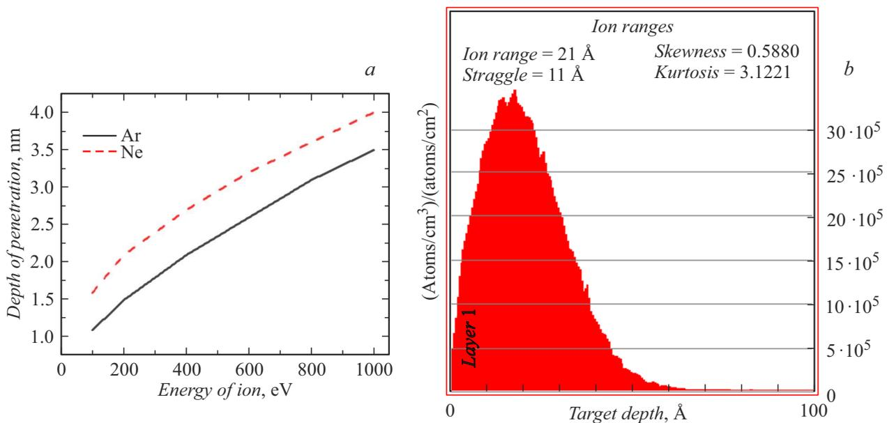
**Figure 5.** *a* — dependence of the penetration depth of Ar and Ne ions on energy; *b* — calculated profile of implanted ions Ne with an energy of 200 eV in the volume of silicon [16].
