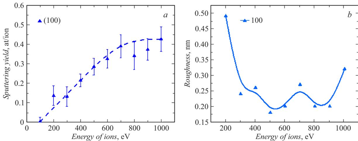
**Figure 1.** The energy dependences of the sputtering yield (a) and the values of the effective roughness (b) of monocrystalline silicon (100).
