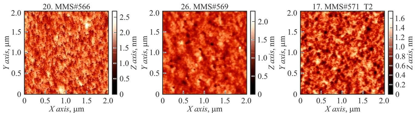
**Figure 4.** AFM frames  $2 \times 2 \mu\text{m}$  surfaces of the main sections of monocrystalline silicon after irradiation with Ne ions with an energy of 100 eV.
