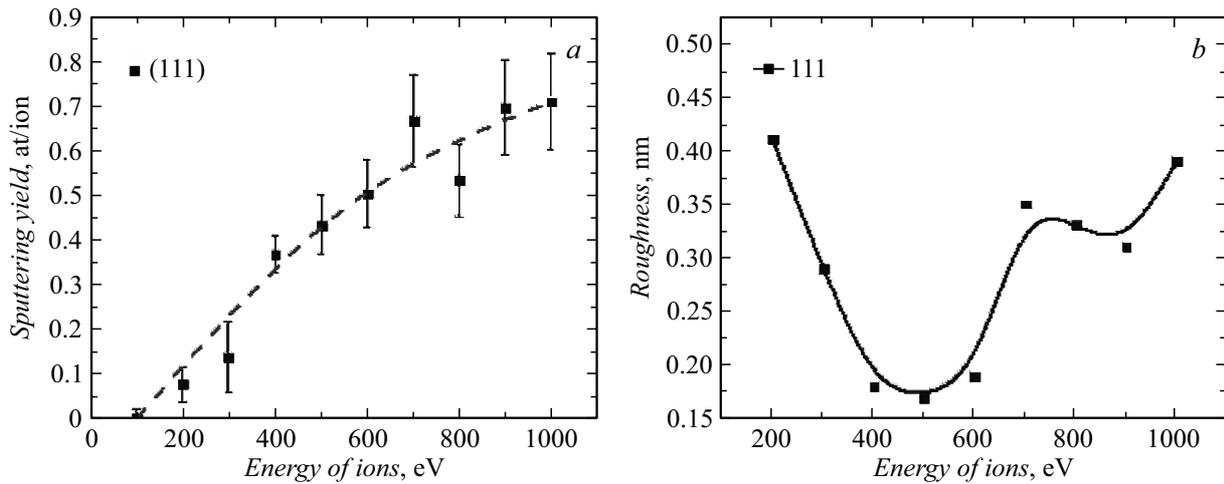
**Figure 3.** The energy dependences of the sputtering yield (a) and the values of the effective roughness (b) of monocrystalline silicon (111).
