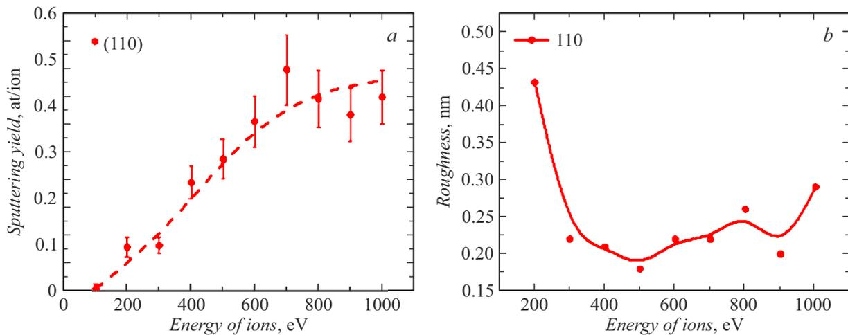
**Figure 2.** The energy dependences of the sputtering yield (a) and the values of the effective roughness (b) of monocrystalline silicon (110).
