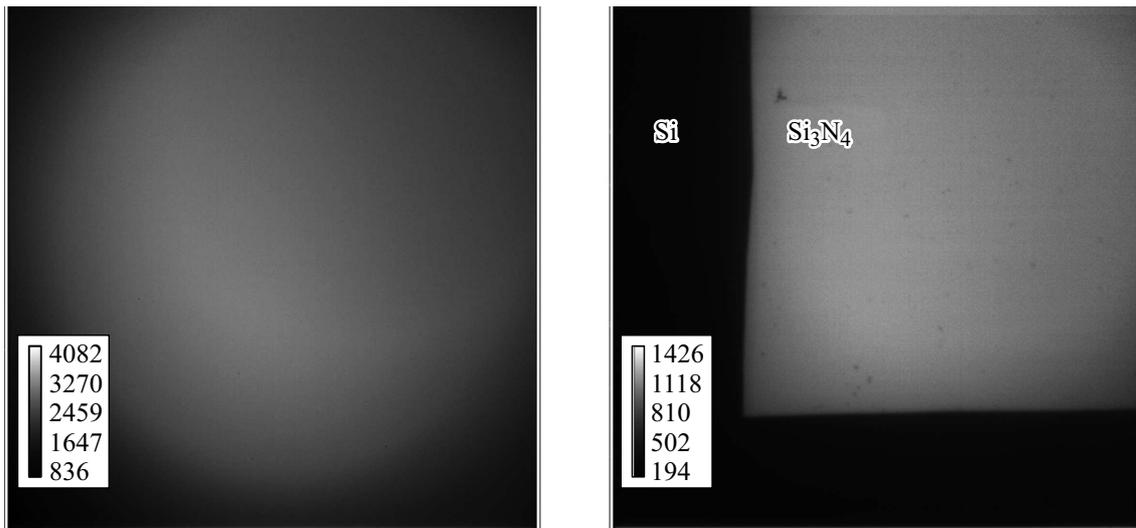
**Figure 4.** Illumination of the field of view of a microscope without a membrane (left) and with a membrane (right).
