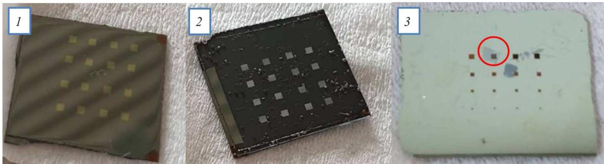
**Figure 3.** The results of some stages of manufacturing. 1 — photoresist with technological pattern; 2 — after ion etching; 3 — final membranes in the plate Si. A sample on the membrane is highlighted in a circle.
