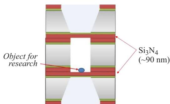
**Figure 6.** Cuvette for living biological samples. The object indicated by the arrow is located between two membranes  $\text{Si}_3\text{N}_4$ .
