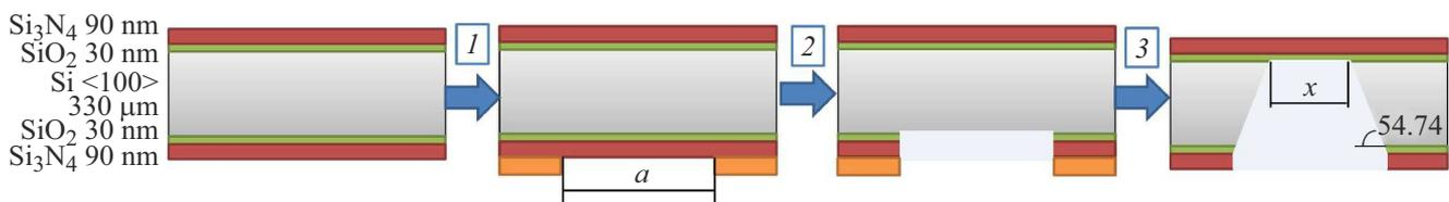
**Figure 2.** Membrane manufacturing scheme  $\text{Si}_3\text{N}_4$ . 1 — applying a photomask to a substrate and creating a technological drawing; 2 — removing layers  $\text{Si}_3\text{N}_4$  and  $\text{SiO}_2$  by ion etching for subsequent chemical etching; 3 — flushing of the photoresist and chemical etching of the remaining Si layer in two stages.
