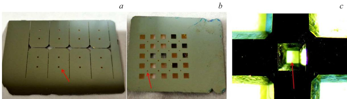
**Figure 5.** Finished membranes after all manufacturing processes using a photomask for contact lithography. The arrows indicate the membranes. *a* — membrane  $0.5 \times 0.5$  mm; *b* — membrane  $0.1 \times 0.1$  mm; *c* — the reverse side of the membrane  $0.1 \times 0.1$  mm.
