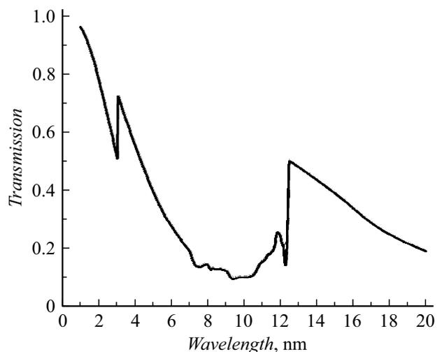
**Figure 1.** Theoretical dependence of the transmission coefficient of the film Si<sub>3</sub>N<sub>4</sub> with a thickness of 90 nm in the range 1–20 nm [8].
