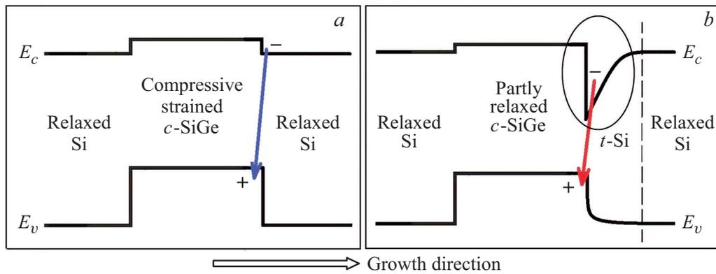
**Figure 2.** Schematic representation of the Si/SiGe/Si heterostructure band diagram in the direction of its growth. *a*) A pseudomorphic section of the structure. *b*) A section with a partially relaxed layer *c*-SiGe and an interfacial QW for electrons (circled by a thin line) in the tensile strained layer *t*-Si on top of it.
