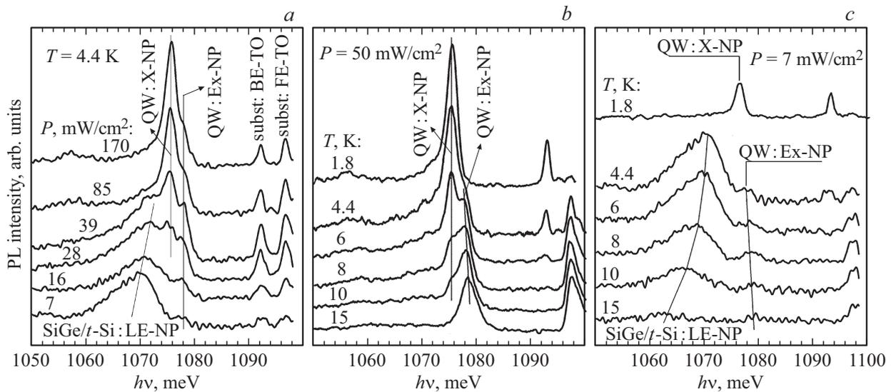
**Figure 4.** Spectra of single-electron no-phonon PL of the studied structure in the NIR region when excited by radiation with a wavelength of  $\lambda_{\text{exc}} = 440 \text{ nm}$ , obtained *a*) at  $T = 4.4 \text{ K}$  and various excitation levels, and *(b, c)* at different temperatures and excitation levels: *b*)  $P = 50 \text{ mW/cm}^2$ , *c*)  $P = 7 \text{ mW/cm}^2$ . The spectra are normalized for the convenience of perception.
