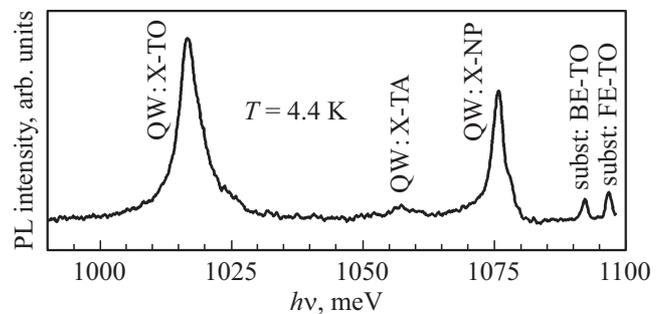
**Figure 3.** Survey spectrum of the PL of the studied structure in the NIR region ( $\lambda_{\text{exc}} = 440 \text{ nm}$ ,  $P = 170 \text{ mW/cm}^2$ ,  $T \approx 4.4 \text{ K}$ ).
