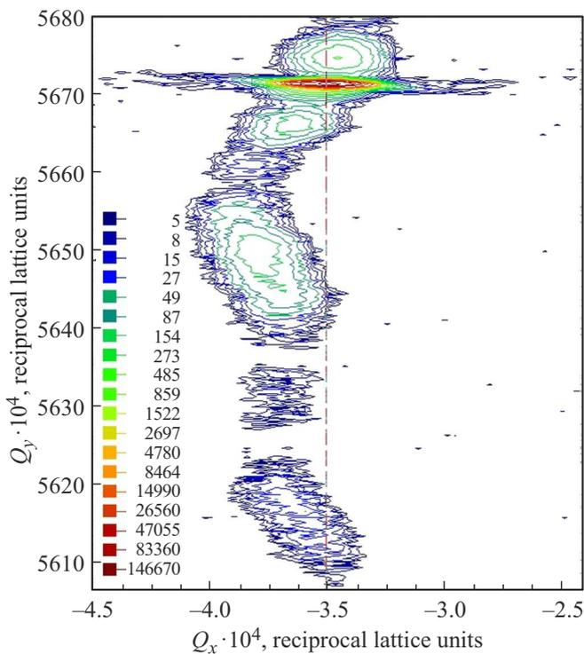
**Figure 1.** Fragment of a two-dimensional region of the reciprocal space [20] near the (004)Si reflection of the structure under study. Continuous contours indicate lines of equal X-ray intensity, and the dashed line corresponds to the center of the substrate peak along the axis  $Q_x$ .
