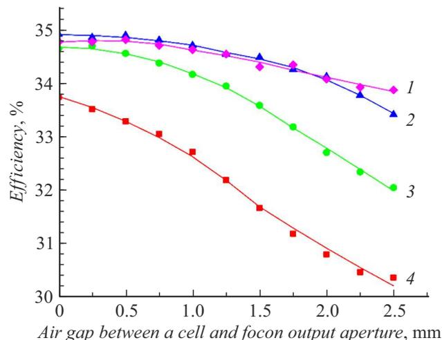
**Figure 5.** Efficiency of radiation conversion in modules with focons with different output aperture sizes vs. size of gap between faces of focon output window and surface of photoreceiving area of solar cell. Output aperture size: 1 — 5 × 5, 2 — 4.5 × 4.5, 3 — 4 × 4, 4 — 3.5 × 3.5 mm.
