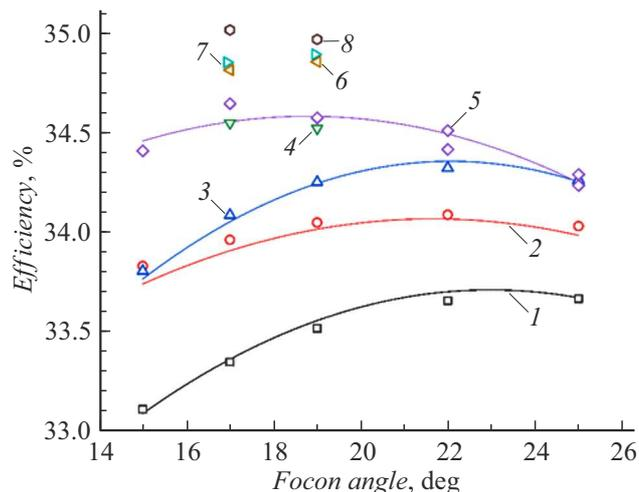
**Figure 3.** Efficiency of radiation conversion in modules with focons of different heights vs. angle of inclination of side faces of focons. Focon height: 1 — 5, 2 — 10, 3 — 15, 4 — 20, 5 — 25, 6 — 30, 7 — 40, 8 — 50 mm.
