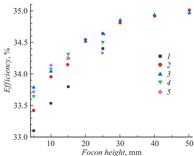
**Figure 4.** Efficiency of radiation conversion in modules with focons with different side face slope angles vs. focon heights. Slope angle: 1 — 15, 2 — 17, 3 — 19, 4 — 22, 5 — 25°.
