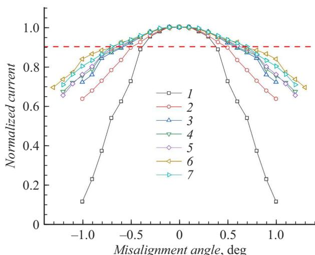
**Figure 6.** Misorientation characteristics of CPM without focon (1) and with installed focons with the corresponding face slope angles and heights: 2 — 19 and 10; 3 — 19 and 15; 4 — 17 and 25; 5 — 19 and 25; 6 — 17 and 40; 7 — 19° and 40 mm. The red dashed line (in the online version) indicates the level above which the concentration of radiation focused on the photoreceiving surface of the solar cell decreases by maximum 10% of the maximum value.
