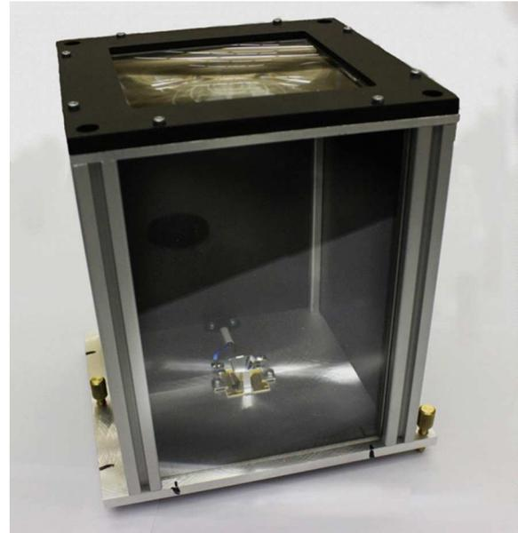
**Figure 2.** External view of CPM with Fresnel lens and focon installed above the photoreceiving area of solar cell.
