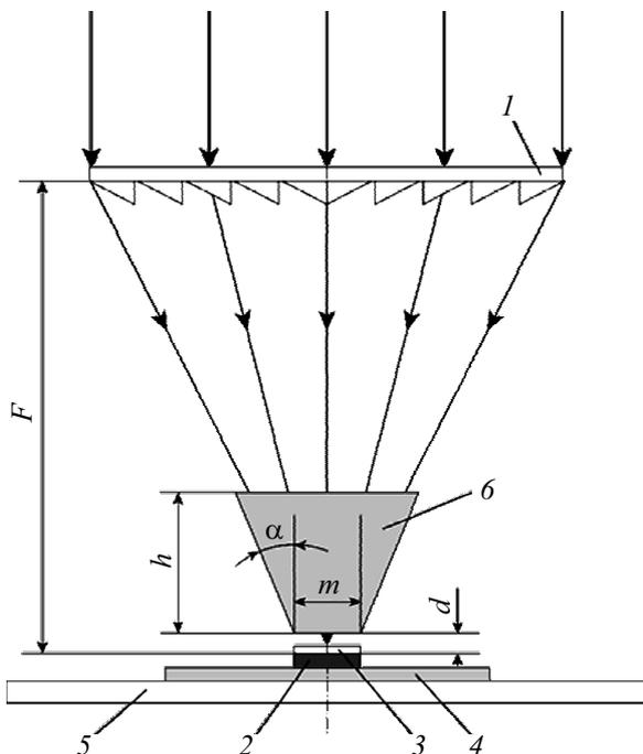
**Figure 1.** Scheme of CPM with secondary concentrator in the form of focon: 1 — Fresnel lens, 2 — solar cell, 3 — protective glass (if available), 4 — heat-conducting electrical insulating board, 5 — aluminum heat-removing base, 6 — focon.  $F$  — focal length of Fresnel lens,  $h$  — focon height,  $m$  — focon output aperture size,  $d$  — gap focon/solar cell,  $\alpha$  — slope angle of focon faces.
