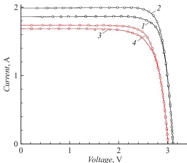
**Figure 7.** CVC of CPM with Fresnel lens with sizes  $120 \times 120$  mm and three-stage GaInP/GaAs/Ge solar cell with sizes  $5.5 \times 5.5$  mm, recorded under irradiation with pulsed simulator: module without focon (1), module with installed focon 40 mm (2) high and recorded when exposed to direct solar radiation: module without focon (3), module with installed focon 40 mm high (4).
