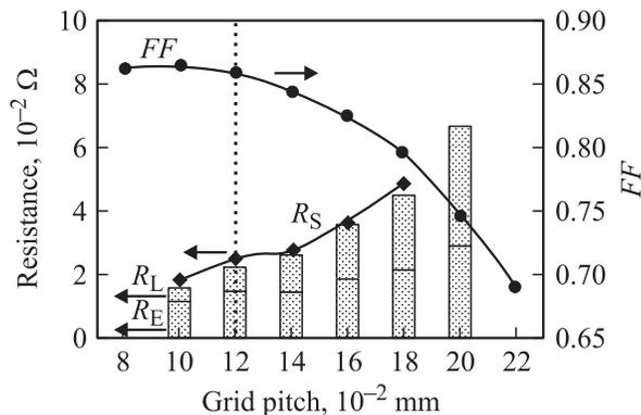
**Figure 3.**  $FF$  of the concentrator cells with various grid pitching under 250-sun light. Series resistance ( $R_S$ ), lateral resistance ( $R_L$ ) and total electrodes resistance ( $R_E$ ) are also shown.
