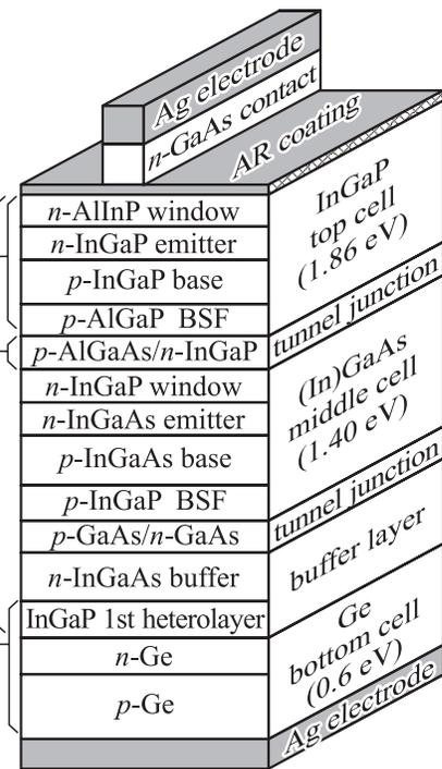
**Figure 1.** Schematic illustration of a triple-junction cell and approaches for improving efficiency of the cell. BSF — back surface field.
