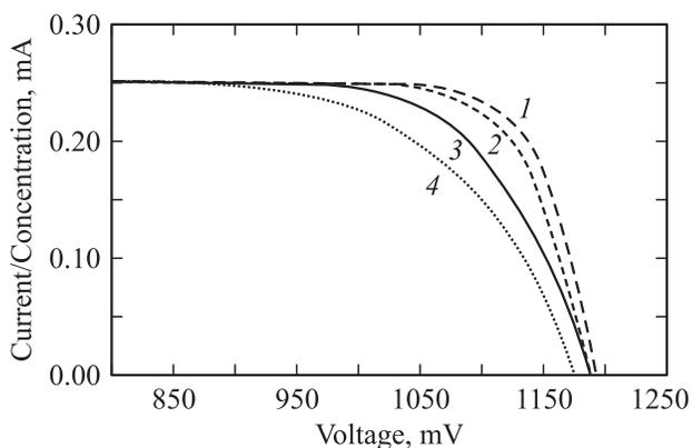
**Figure 3.** Illumination *I-V* curves of the concentrator solar cell considering the four cases covered in figures 1 and 2, illumination 1000 suns average: 1 and 2 — good quality front contacts, 3 and 4 — medium quality front contact, 1 and 3 — uniform illumination, 2 and 4 — non-uniform illumination.
