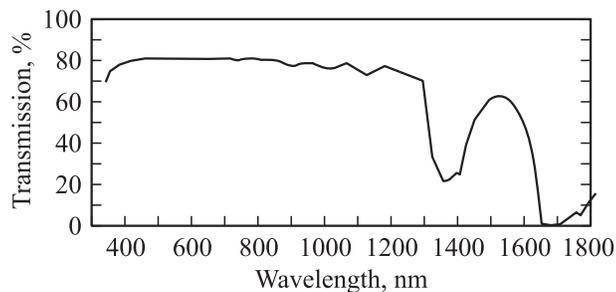
**Figure 4.** Spectral transmission of the TIR-R concentrator like the one described in [18].
