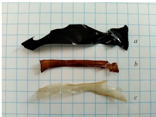
Figure 1. Stretched PVA-iodine (a), initial, (b) partly and (c) nearly completely deiodinated films.
