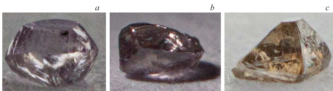
Figure 2. Specimen photos. a — specimen № 1, pink, one polished surface, 14 mg; b — sample № 2, pink, dodecahedral habit, 16 mg; c — specimen № 3, brown, 20 mg, octahedral habit.
