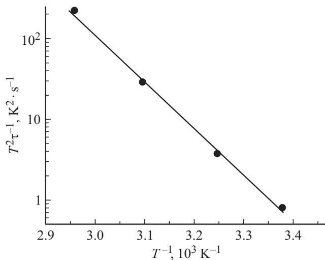
**Figure 3.** Arrhenius law for degradation of an Ag/SnSe/Ge<sub>2</sub>Se<sub>3</sub>/W SDC memristor in the 22–65°C temperature interval. The activation energy is 1.16 eV.
