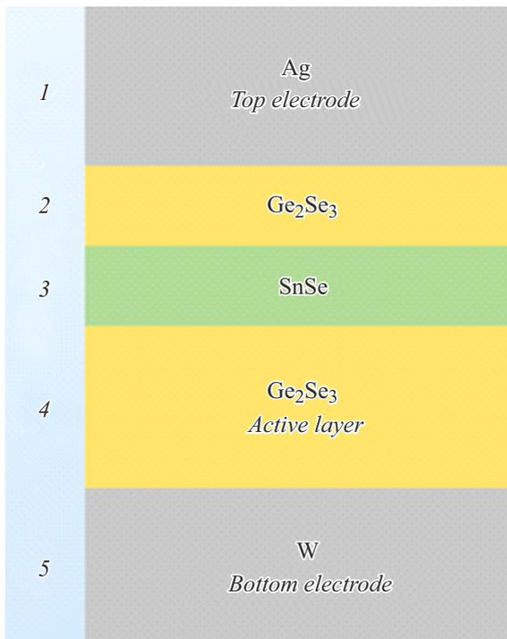
**Figure 1.** Sequence of layers and their functionality in an Ag/SnSe/Ge<sub>2</sub>Se<sub>3</sub>/W SDC memristor. 1 — active silver electrode, 2 — spacer, 3 — Sn ion source, 4 — solid Ge<sub>2</sub>Se<sub>3</sub> electrolyte (active layer), 5 — inert tungsten electrode. The interelectrode space is 15 nm.
