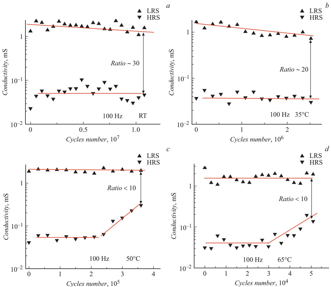
**Figure 2.** Degradation curves for LRS and HRS at temperatures of 22 (a), 35 (b), 50 (c), and 65°C (d) measured within 30, 7, 1, and 0.142 h, respectively.
