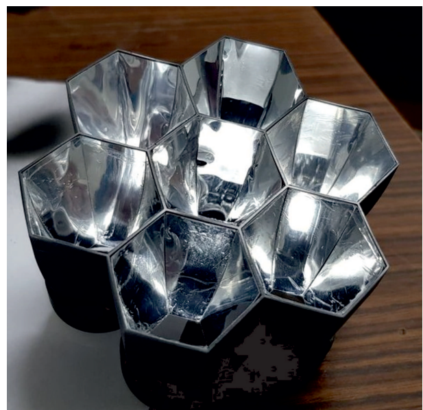
Figure 2. Prototypes of Winston hexagonal cones with a reflective film applied to the inner surface.
