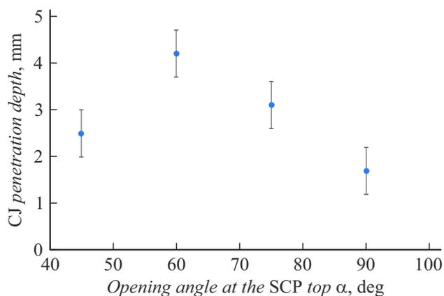
**Figure 3.** Dependence of the depth of CJ penetration into the steel obstacle on the value of the angle at the apex CEM. Samples of copper grade M0b.
