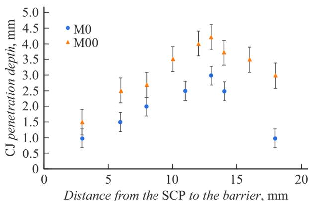
**Figure 4.** Dependence of the CJ penetration depth in the steel barrier on the distance from the CEM to the barrier for copper samples of M0b and M00k grades.
