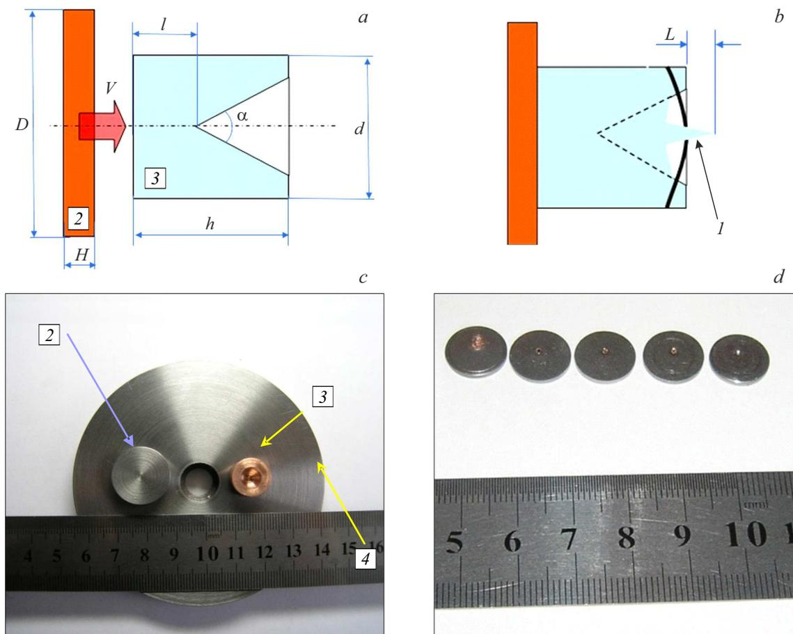
**Figure 1.** Schematic of the experiment using the cumulative indentation sample: *a* — the sample geometry before impact, *b* — the formation of CJ in the sample after impact, *c* — equipment, projectile and copper sample before test, *d* — 5 punched targets with thickness 1 mm after test. *l* — CJ, *2* — projectile, *3* — sample, *4* — tools.
