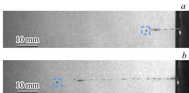
**Figure 2.** High-speed jet shooting. The scheme of the experiment is shown in Fig. 1. No steel barrier was installed during the shooting, and the jet was free to stretch out to destruction. The CJ head element is marked with a dotted line. The interval between frames *a* and *b* is 16  $\mu$ s.
