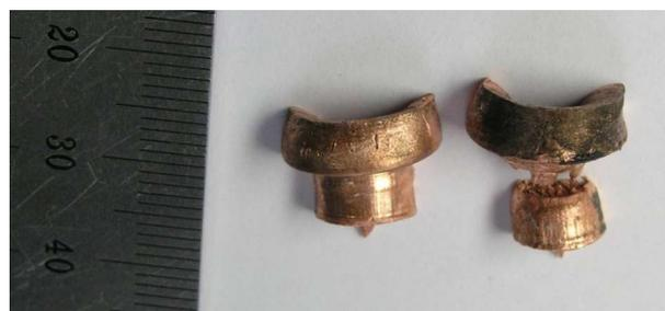
**Figure 5.** Photos of CEM after tests. To the left — sample of copper grade M0b, to the right — sample of copper grade M00k.
