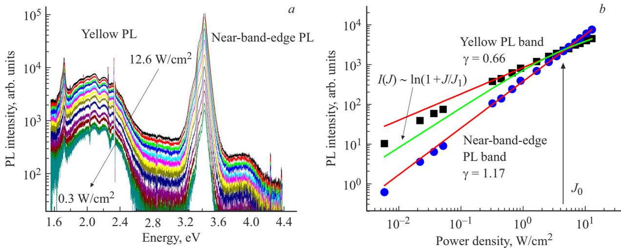
**Figure 4.** PL GaN spectra (a) and the dependences of the intensity of the edge and yellow PL bands (b) on the power of excitation at 300 K. The solid lines show the approximation by the exponential function of the kind  $I(J) \sim J^\gamma$  for the both PL bands and by the logarithm of the kind  $I(J) \sim \ln(1 + J/J_1)$  for the yellow PL band. (A color version of the figure is provided in the online version of the article).
