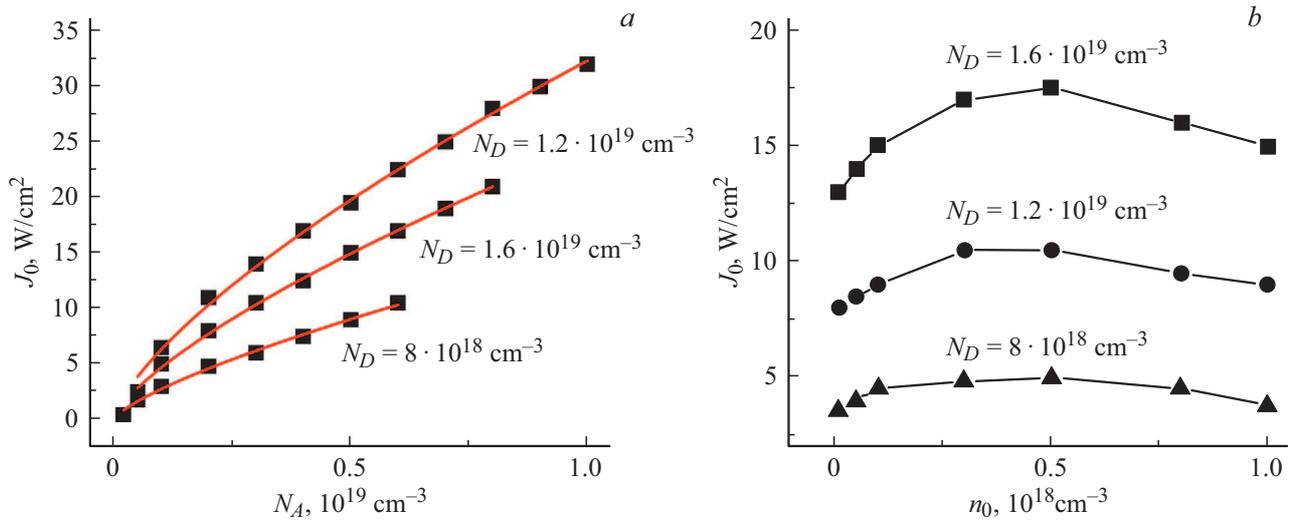
**Figure 3.** Calculation of the density of the density of the power of excitation  $J_0$ , at which the rates of recombination of the  $BB$  and  $DA$  channels, for  $N_D = 8 \cdot 10^{18}$ ,  $1.2 \cdot 10^{19}$  and  $1.6 \cdot 10^{19} \text{ cm}^{-3}$ :  $a$  — on the concentration of the acceptors  $N_A$  at  $n_0 = 3 \cdot 10^{17} \text{ cm}^{-3}$ ,  $b$  — on  $n_0$  at  $N_A/N_D = 0.25$ .
