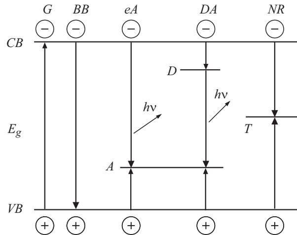
**Figure 1.** Diagram of the transitions in the compensated semiconductor in interband generation of the charge carriers.
