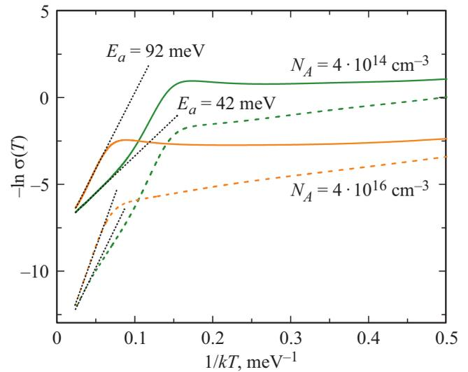
**Figure 3.** Calculated dependences of the logarithm of the values  $\sigma$  (solid lines) and  $\sigma/T^{3/2}$  (dotted lines) on the temperature for the CHT film with 22% of cadmium at different concentrations of mercury vacancies  $N_A$ . The donor concentration is fixed and equal to  $2 \cdot 10^{14} \text{ cm}^{-3}$ . It was assumed in the calculation that  $\mu_n/\mu_p = 200$ .
