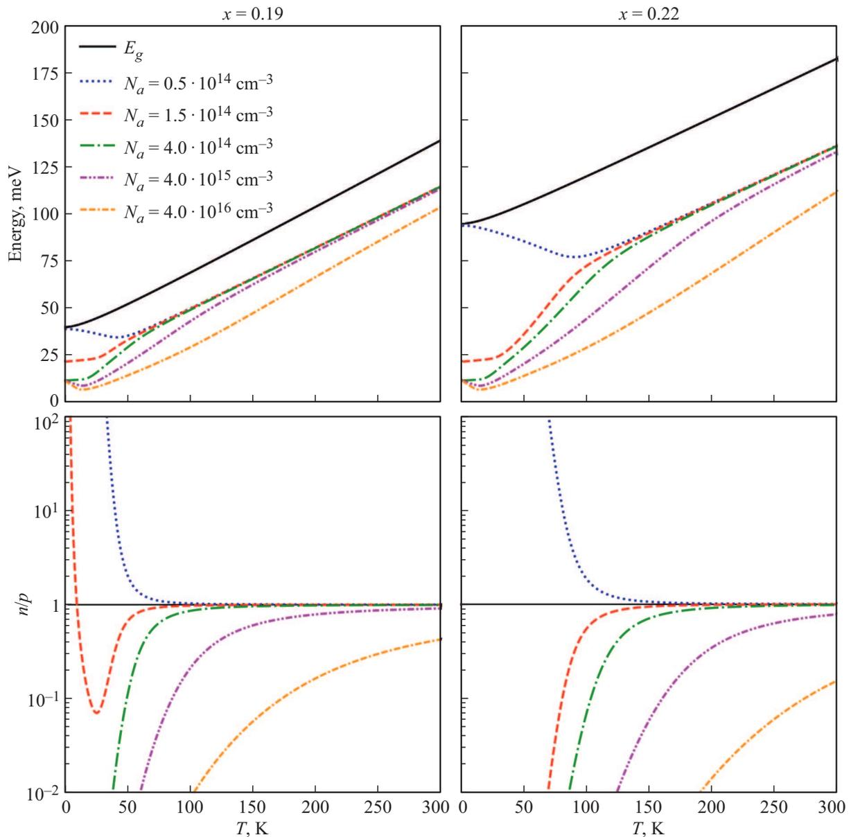
**Figure 2.** Calculated dependence of the Fermi level position and the relative concentration of electrons and holes on temperature at various degrees of compensation of mercury vacancies by donors. The donor concentration is fixed and equal to  $2 \cdot 10^{14} \text{ cm}^{-3}$ . (Colored version of the figure is presented in electronic version of the article).
