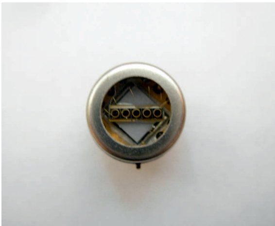
Figure 2. Photodiode array of 5 elements in standard package TO-8.
