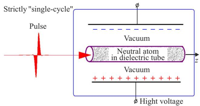
**Figure 1.** Scheme of experiment and main idea. The gas tube is placed in DC external electric field. A single-cycle laser pulse runs through the tube ionizing the electrons.
