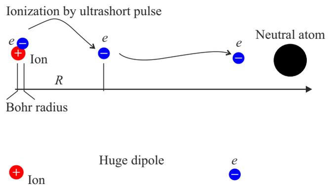
**Figure 2.** Schematic description of the three-step generation mechanism of unipolar terahertz pulse — the appearance of the free electron due to ionization, leading to the occurrence of a giant dipole. The subsequent electron acceleration by the DC external field and its annihilation upon collision with a wall or another atom.
