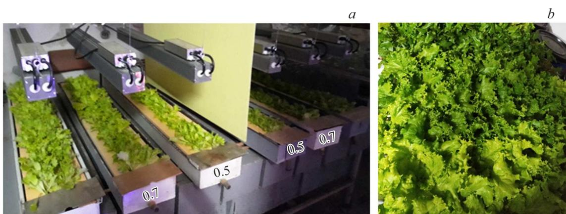
**Figure 2.** General view of experimental vegetation lighting systems with lettuce plants: *a* — under LED light sources, *b* — under HPS lamps.
