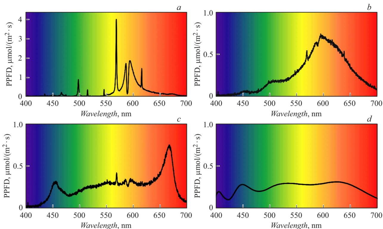
**Figure 1.** Emission spectra of light sources: *a* — HPS, *b* — LED1 (yellow light), *c* — LED2 (pink light), *d* — LED3 (close-to-sunlight).
