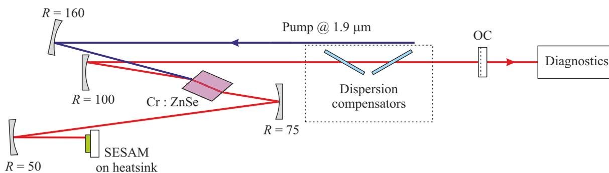
**Figure 1.** Scheme of passively mode-locked Cr:ZnSe laser.
