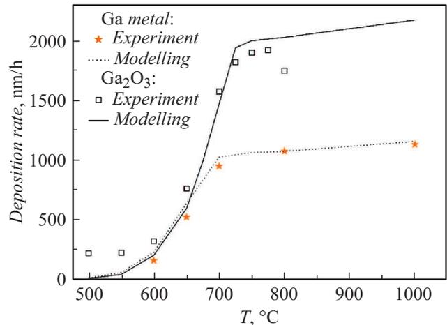
**Figure 3.** Comparison between the temperature dependences of experimental (symbols) and calculated (curves) deposition rates of metallic gallium and Ga<sub>2</sub>O<sub>3</sub> (nitrogen is the carrier gas).
