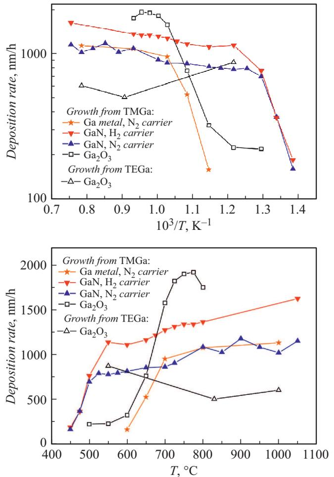
**Figure 1.** Temperature dependences of the deposition rate of Ga<sub>2</sub>O<sub>3</sub>, GaN, and metallic gallium plotted in different coordinates.
