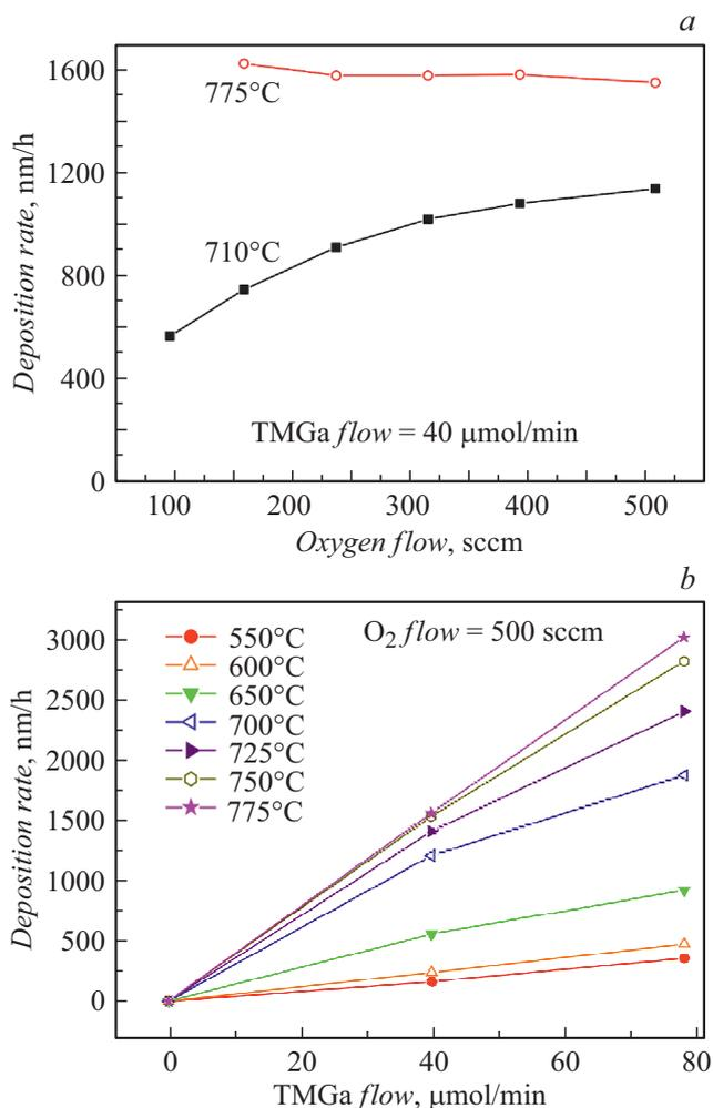
**Figure 2.** Dependences of the deposition rate of Ga<sub>2</sub>O<sub>3</sub> on the flow of oxygen (a) and TMGa (b) at different temperatures.
