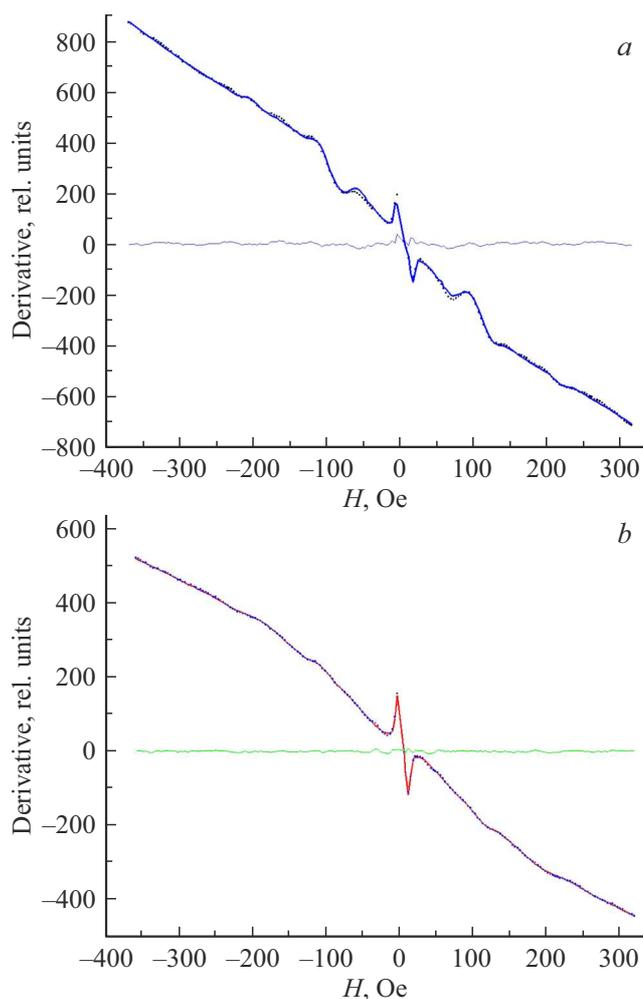
**Figure 3.** Experiment 3. LF 725 nm, neon-20,  $p < 0.1$  Torr,  $i = 29$  mA. Horizontal curve — deviations of the experimental diagram from the model curve („residuals“). *a*) OMFCRs, centered on 10, 90, 110, 200 Oe, deviation 17 Gs, 16 passes; *b*) OMFCRs, centered on 10, 110 and 200 Oe, deviation 10 Gs, 28 passes.
