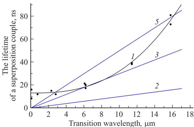
**Figure 6.** Dependence of the interference duration of isotope pair atoms on the transition wavelength: 1 is an experimental dependence described by the function  $T_{\text{int}} = 13.144 + 0.046\lambda^{2.455}$ ; 2–5 — times of isotope atom scattering to a distance  $\lambda$  in the direction orthogonal to the pair axis due to multidirectional atoms motion with velocities  $\langle V_i \rangle$ ,  $1/3\langle V_i \rangle$ ,  $1/5\langle V_i \rangle$  respectively.
