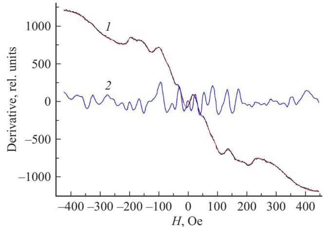
**Figure 2.** Experiment 2. 1 — OMFCRs, centered on 50, 130, 200, 240 and 280 Oe. Neon-20,  $p \sim 0.1$  Torr,  $i = 30$  mA, deviation 12 Gs, IRLF LF-7, 3 passes. 2 — deviations of the experimental diagram from the model curve increased by a factor of 10 („residuals“).
