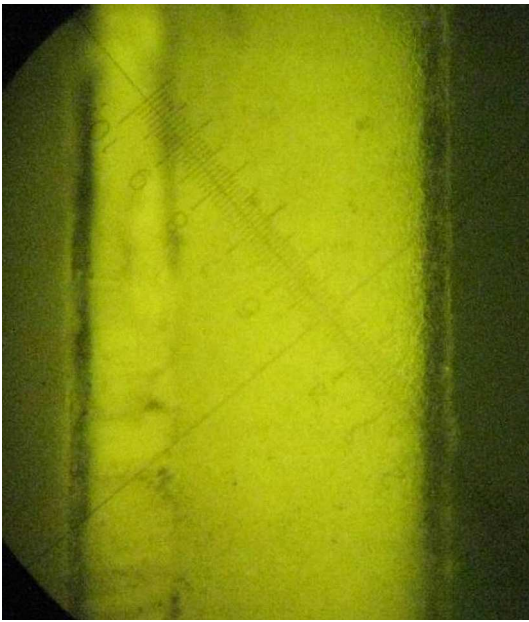
Figure 4. Photo of the sample end luminescence at 300 K after Be diffusion, 2100°C, 2 h. A 80 \mu\text{m} dark near-surface layer can be seen. Sample thickness is 1700 \mu\text{m} .
