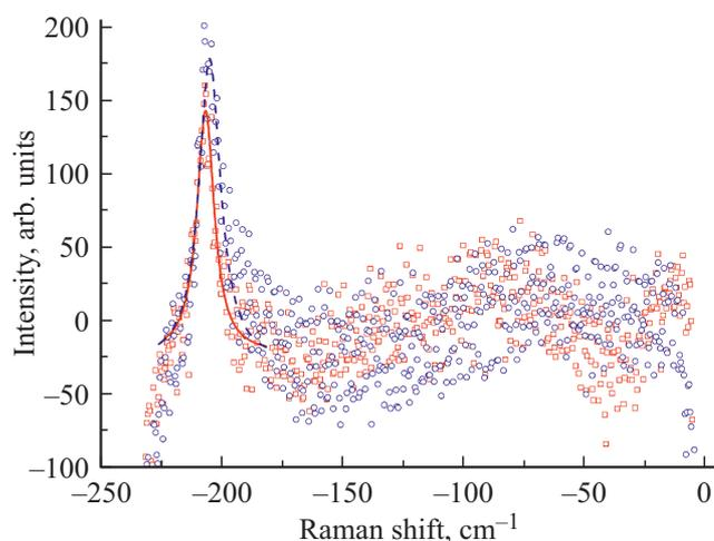
**Figure 2.** RS spectra (anti-Stokes component; after background subtraction) for QDs CdSe/CdS/ZnS on glass substrate (red squares) and QDs embedded in PIB (blue circles) measured at room temperature. The solid and dashed lines show the results of data approximation by the Lorentz function.
