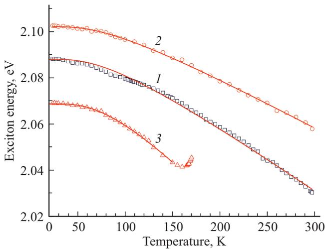
**Figure 1.** Temperature dependences of the maximum position of the luminescence spectrum (exciton energy) for nanocomposites based on QDs CdSe/CdS/ZnS deposited on the surface of glass substrate (1), embedded in PIB (2), embedded in frozen toluene (3) and their approximation (solid lines) using formula (2).
