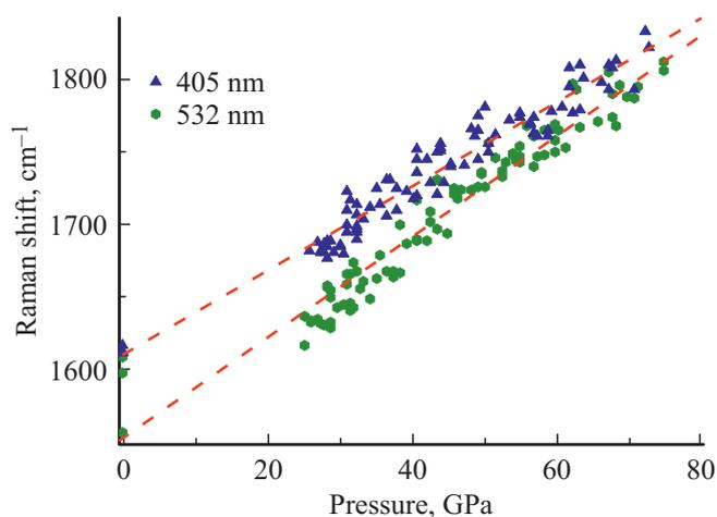
**Figure 4.** Dependence of the Raman frequency of 3D  $C_{60}$  on pressure. Spectra were measured at a laser power of 15 mW, the measurement time was 10 min, and the excitation radiation wavelengths were 405 nm (triangles) and 532 nm (circles).
