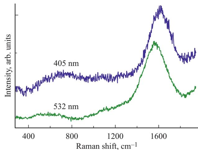
**Figure 2.** Raman spectra of the 3D  $\text{C}_{60}$  sample. Spectra obtained prior to unloading were measured at a laser power of 1 mW. The measurement time was 10 min, and the excitation radiation wavelengths were 405 and 532 nm.
