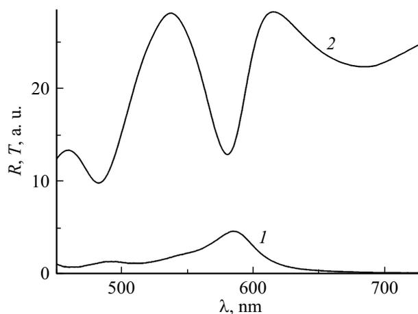
**Figure 2.** Transmission (1) and reflection spectra (2) of a hybrid Ag/SiO<sub>2</sub>/Ag/ML/Ag plasmon-photonic crystal with the light incidence angle  $\theta = 16^\circ$ .
