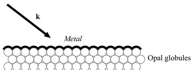
**Figure 1.** Use of the periodic texture at the metal–dielectric interface for SPP excitation ( $\mathbf{k}$  — wave vector of the incident electromagnetic wave) [29].
