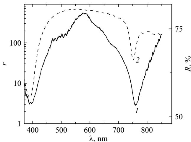
**Figure 4.** Spectral dependence of  $r = T_3(\lambda)/(T_1(\lambda)T_2(\lambda))$  (1) ratio and reflection spectrum  $R(\lambda)$  of Ag/SiO<sub>2</sub>/Ag resonator (2). Light incidence angle  $\theta = 16^\circ$ .
