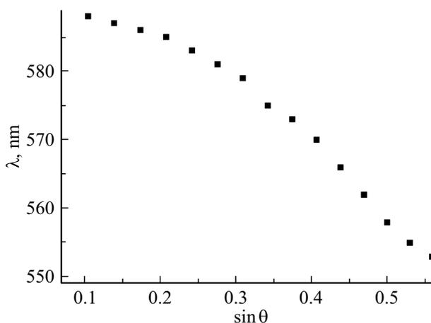
**Figure 3.** Angular dispersion of the spectral position of the long-wave maximum of EOT for the hybrid Ag/SiO<sub>2</sub>/Ag/ML/Ag plasmon-photonic crystal.
