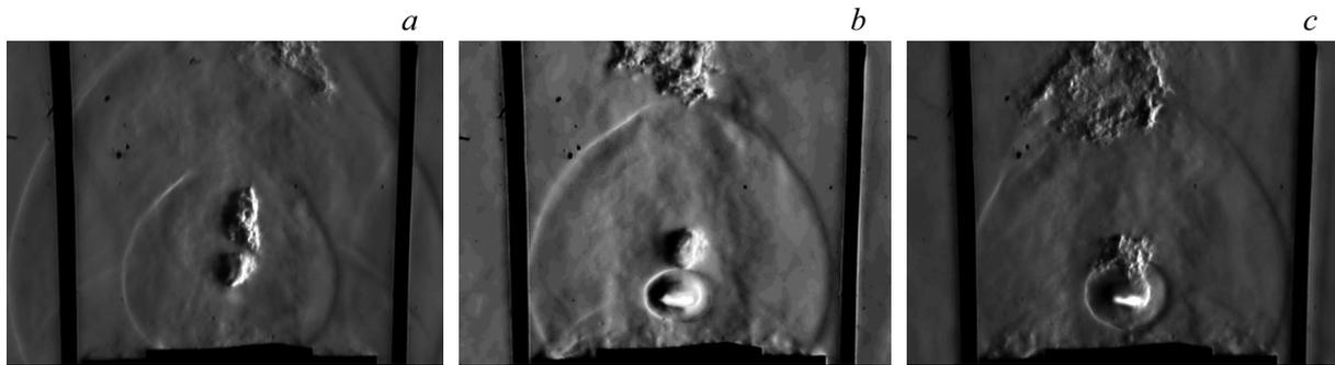
**Figure 4.** Shadow recording for the case with two plane electrodes in a subsonic flow: *a* — when an electric field is absent; *b* — field (6 kV) is directed from left to right; *c* — field is directed from right to left.
