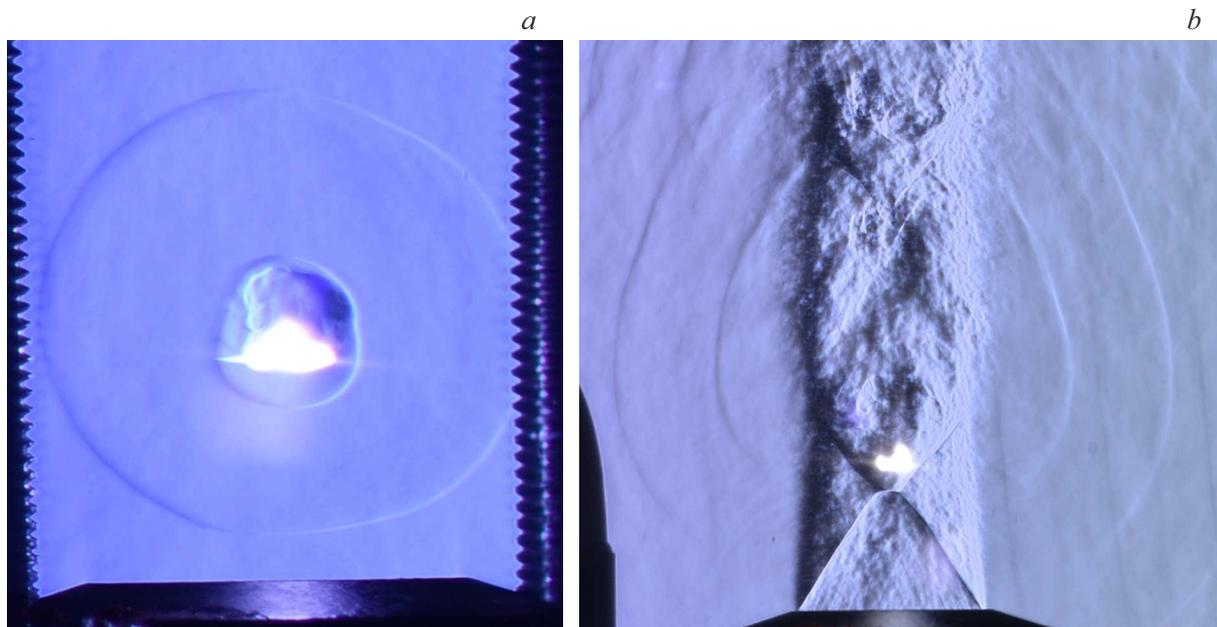
Figure 3. Shadow recording of an optical discharge when an electric field is absent: *a* — without a flow; *b* — in a supersonic flow ( $P_0 = 0.66$  MPa).
