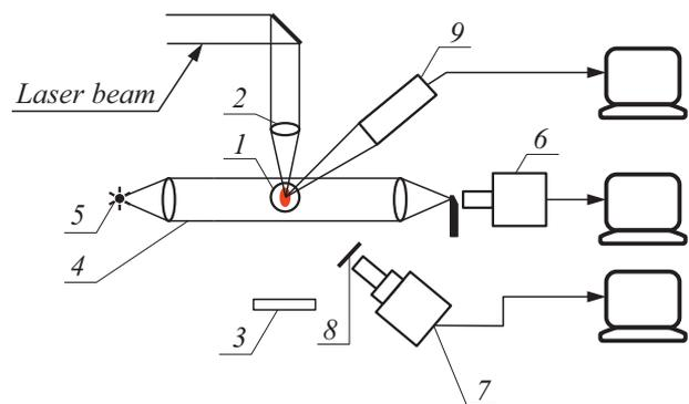
**Figure 1.** Experiment layout: 1 — object under observation; 2 — lenses; 3 — absorber; 4 — schlieren system; 5 — light source; 6 — photocamera; 7 — high-speed camera; 8 — interference filter; 9 — CCD-camera.
