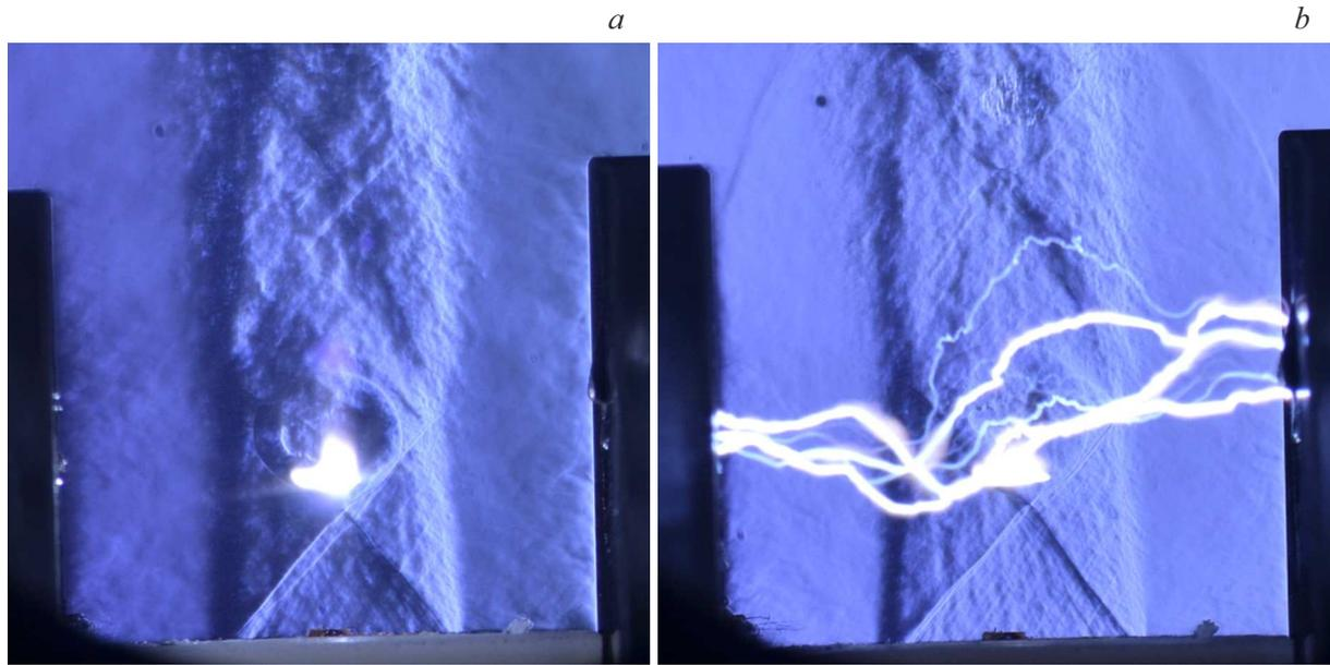
**Figure 6.** Optical discharge in a supersonic jet when an electric field is present (total pressure  $P_0 = 0.5$  MPa,  $U = 22$  kV): *a* — without streamers, *b* — with streamers.
