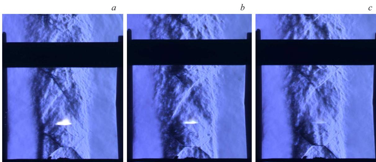
**Figure 7.** Quenching of optical discharge at an increase in electric field intensity (from left to right), the field being across the beam ( $P_0 = 0.3 \text{ MPa}$ ,  $U = 11\text{--}22 \text{ kV}$ ).
