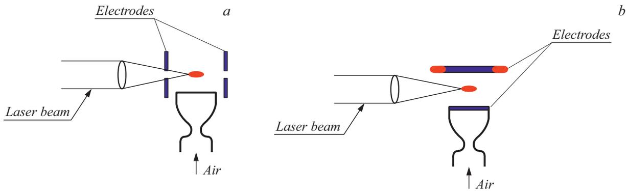
Figure 2. Layout of the electrodes and laser beam: *a* — electric field along the beam; *b* — field across the beam.
