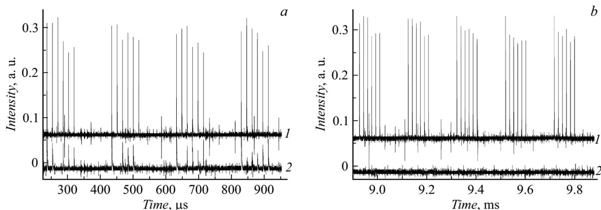
**Figure 8.** Photometric recording of radiation at quenching of an optical discharge.
