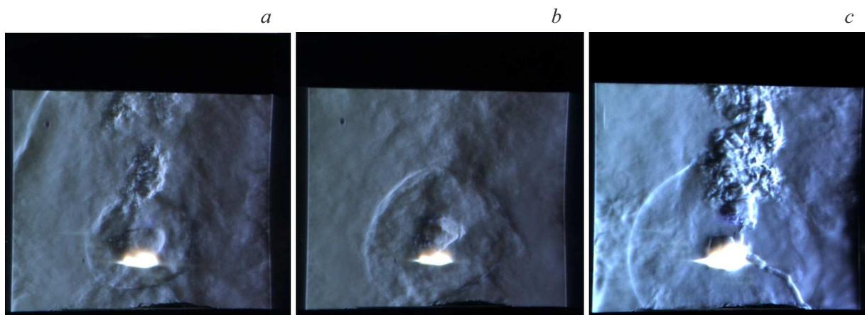
**Figure 5.** Shadow recording for the case of circular electrodes (the anode is above) in a subsonic flow: *a* — without an electric field ( $\Delta p = 0.6$  atm); *b* —  $U = 18.5$  kV ( $\Delta p = 0.6$  atm); and *c* —  $U = 18.5$  kV,  $\Delta p = 0.016$  atm.
