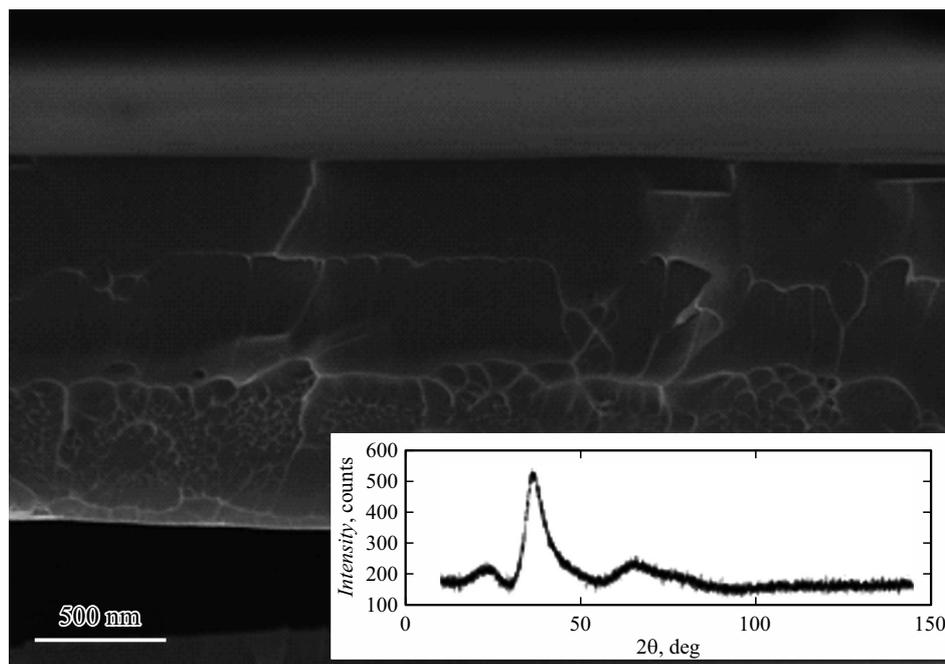
**Figure 1.** The surface and transverse fracture of the Pt : Zr = 1 : 4 amorphous film applied on a flat substrate, and its diffraction pattern (in the inset).
