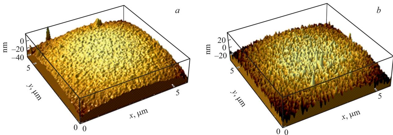
**Figure 3.** Surface reliefs of the films obtained on microspheres at different discharge powers: a — 50 W (amorphous), b — 140 W (crystalline).
