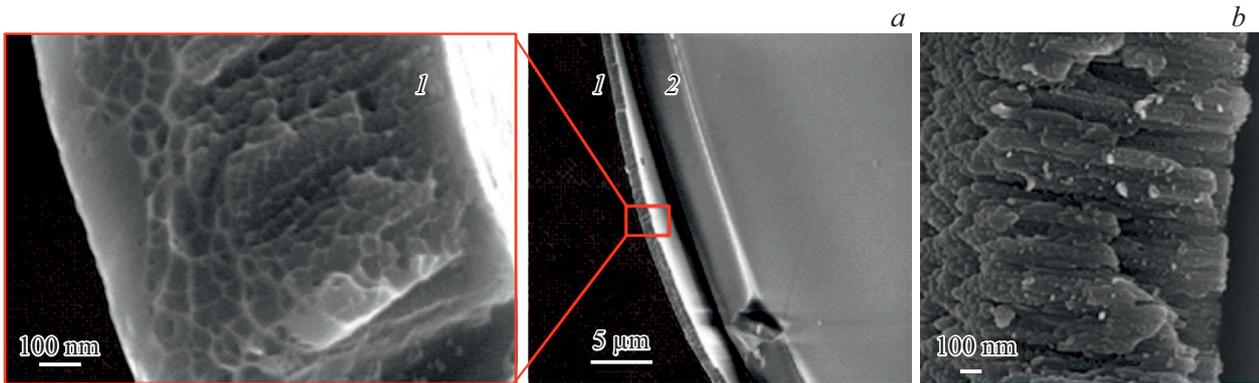
**Figure 2.** The fracture images of the amorphous metal film (a) and crystalline film of the same composition (b) on the spheres 0.5 mm in diameter. 1 — film fracture, 2 — spherical substrate fracture.
