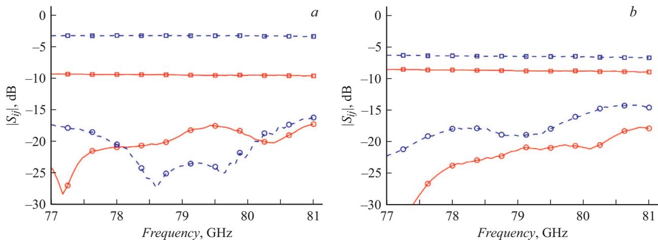
**Figure 2.** Modules of reflection  $S_{11}$  (circles), transmission  $S_{21}$  (squares) coefficients for coplanar lines 61.35 mm long (solid line) and 18.85 mm long (dashed line) (a), and for microstrip lines 43 mm long (solid line) and 21 mm long (dashed line) (b).
