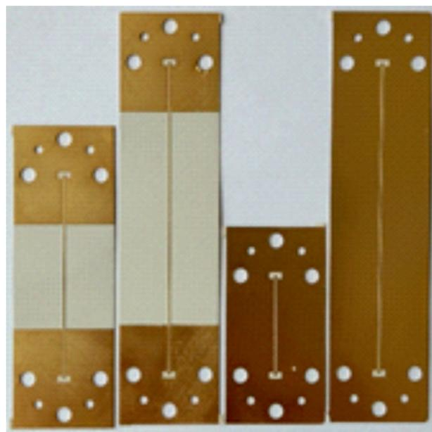
**Figure 1.** The transmission lines under study are: microstrip lines (left) and coplanar lines (right).
