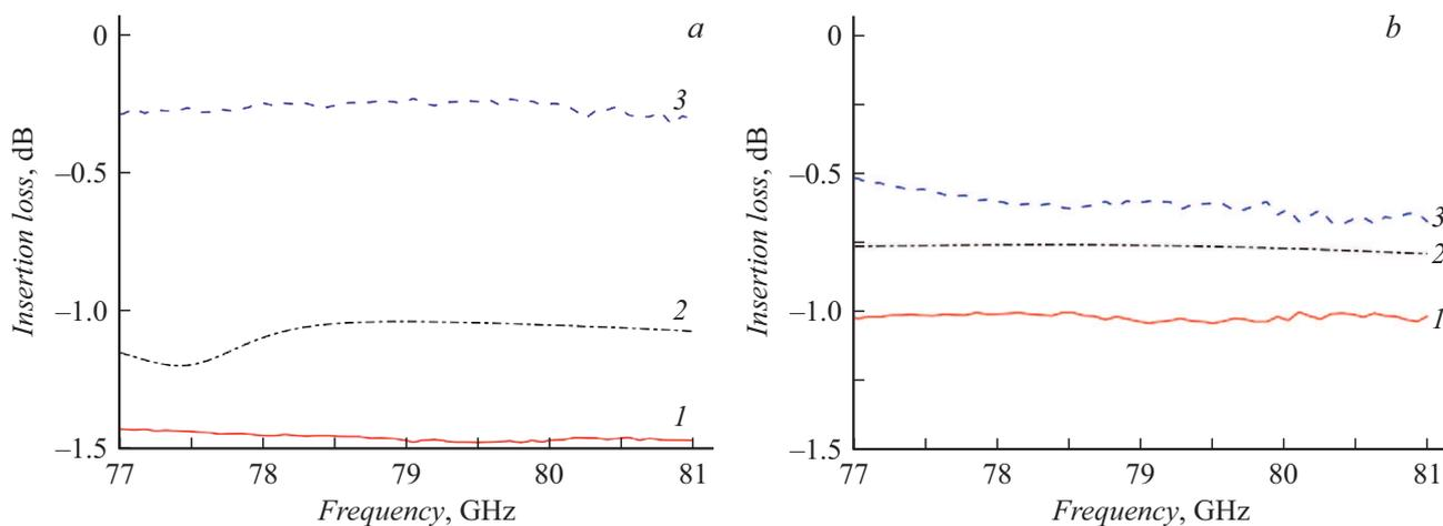
**Figure 3.** Inserted loss in the 10 mm coplanar line section determined experimentally (1), by simulation (2), and in the waveguide–coplanar line junction (3) (a), and that in the 10 mm microstrip line section determined experimentally (1), by simulation (2) and in the coplanar–microstrip line junction (3) (b).
