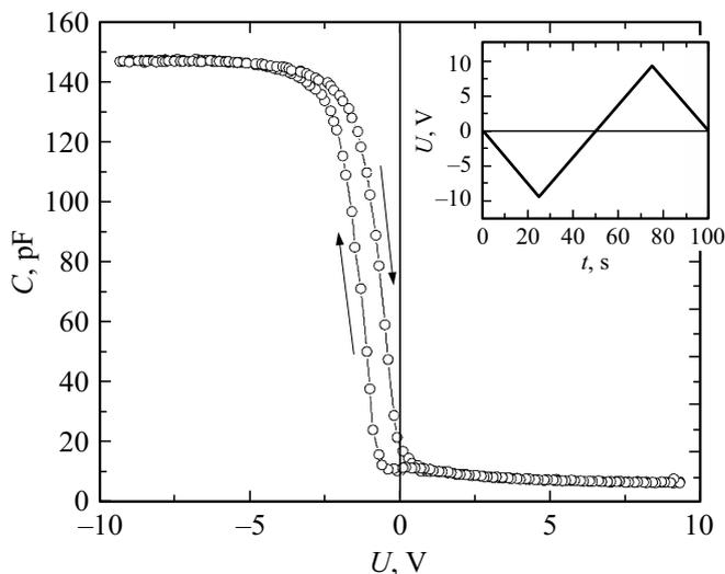
**Figure 3.** The room-temperature  $C(U)$  dependence for heterostructure Al/Cr/SBN-50/BST-20/Si(001)/Cr/Al. The inset presents the  $U(t)$  dependence.
