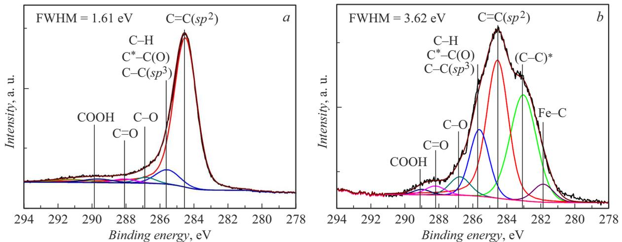
**Figure 2.** XPS C 1s spectra. a — initial MWCNTs, b — plasma treated MWCNTs.
