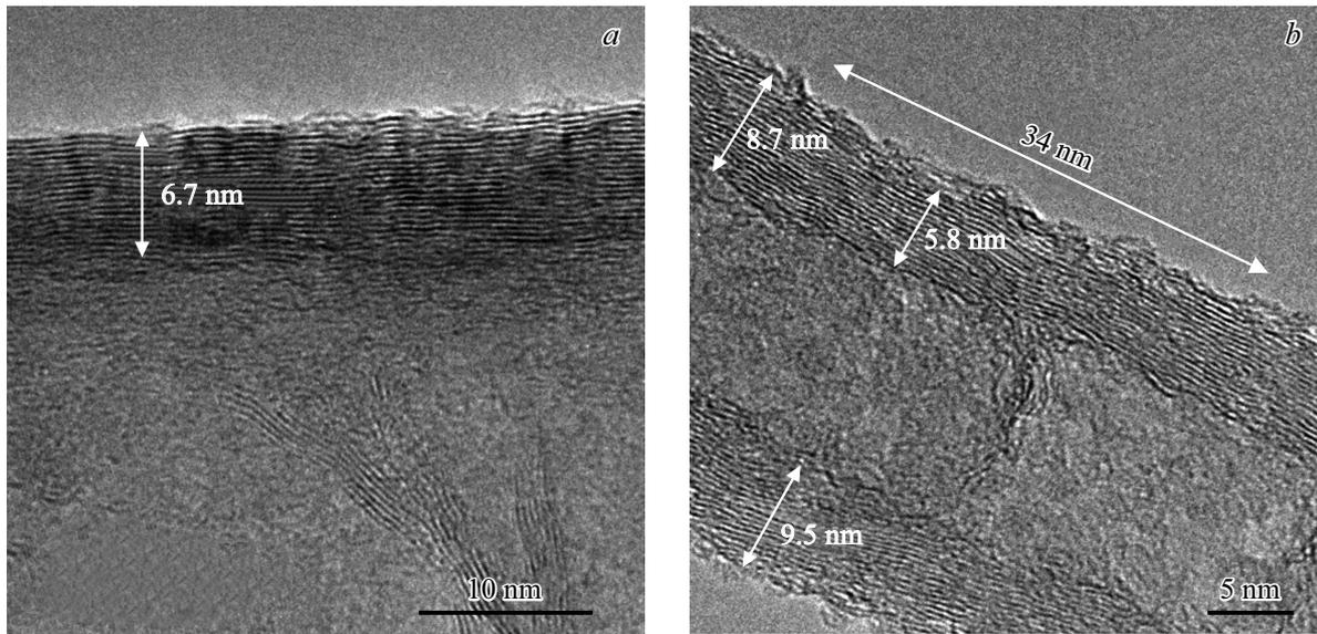
**Figure 1.** TEM image of the MWCNT wall prior to plasma treating (a) and of MWCNT after plasma treating (b).
