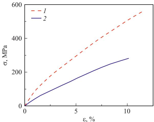
**Figure 1.** Stress-strain curves for high-strength oriented mono- (1) and polyfilament PP fibers (2).
